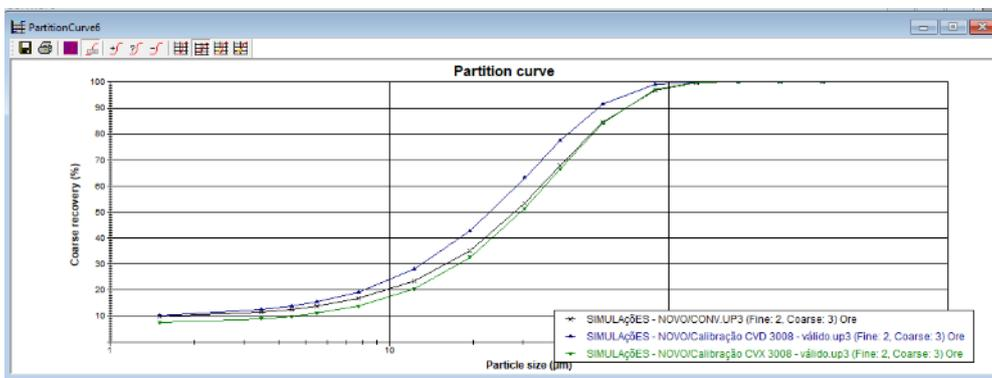
Figure 7 – CVX cyclone cluster simulation changing vortex to 155mm.
