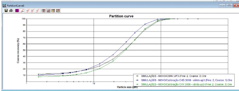
Figure 6 – CVX cyclone battery simulation changing apex to 100mm.
