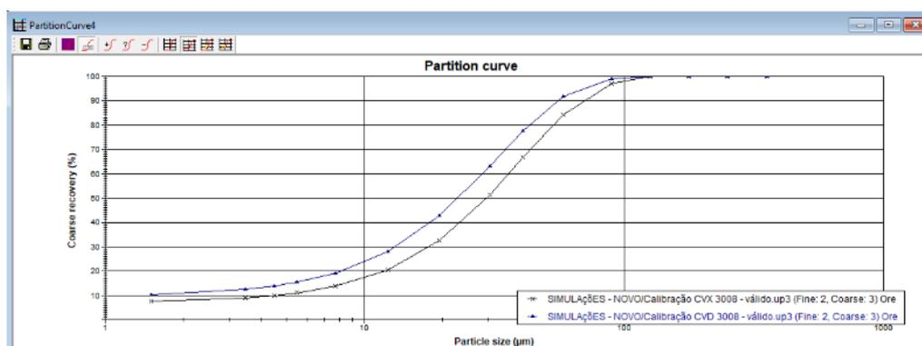
**Figure 5** – Comparison of CVX versus CVD partition curves.**Table 3** – Mass recovery for the 1st desliming stage VGR2.
