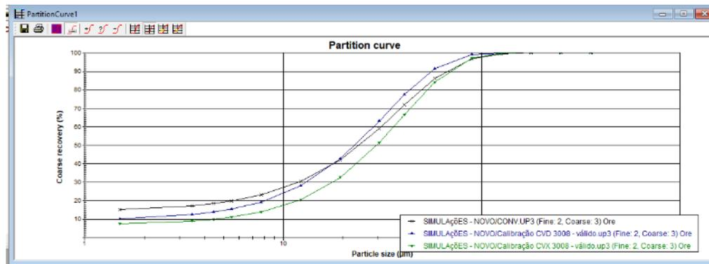
**Figure 8** – CVX cyclone cluster simulation changing apex to 100mm and vortex to 155mm.
