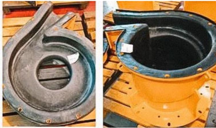
Figure 3 – The lid (left) and the chamber (right) modules.
