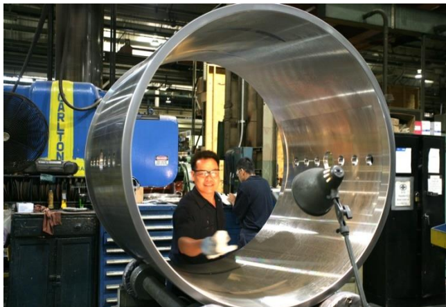
Figure 9 — Final inspection of a dual pad bushing prior to shipping
