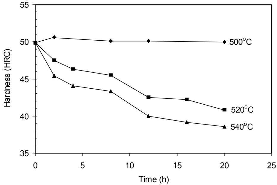
Figure 3. Aging behaviour at 500, 520 and 540°C for samples previously double tempered at 520°C.
