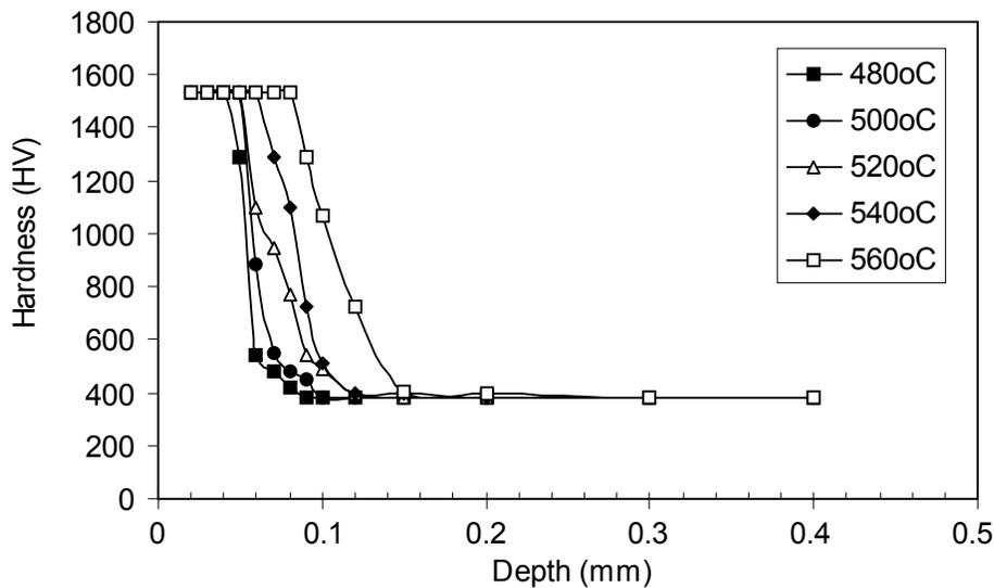
Figure 7. Hardness profiles determined after plasma nitriding, 4 hours, for a substrate tempered at 580°C.
