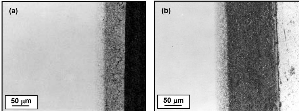
**Figure 5.** Surface microstructures observed on optical microscopy after nitriding at (a) 480°C and (b) 560°C. Etch: Nital 10%.
