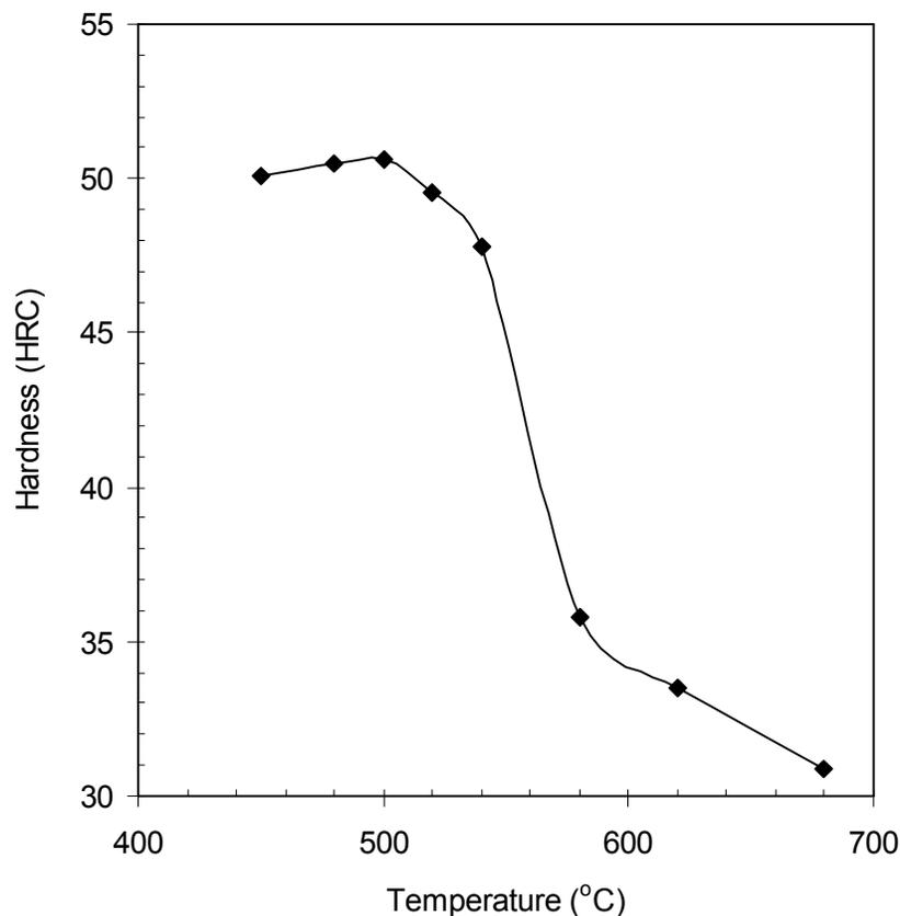
**Figure 1.** Tempering curve for the martensitic stainless steel type AISI 420.
