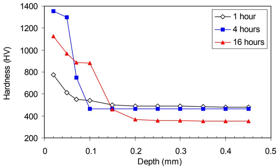
**Figure 2.** Hardness profiles determined after plasma nitriding at 520°C.
