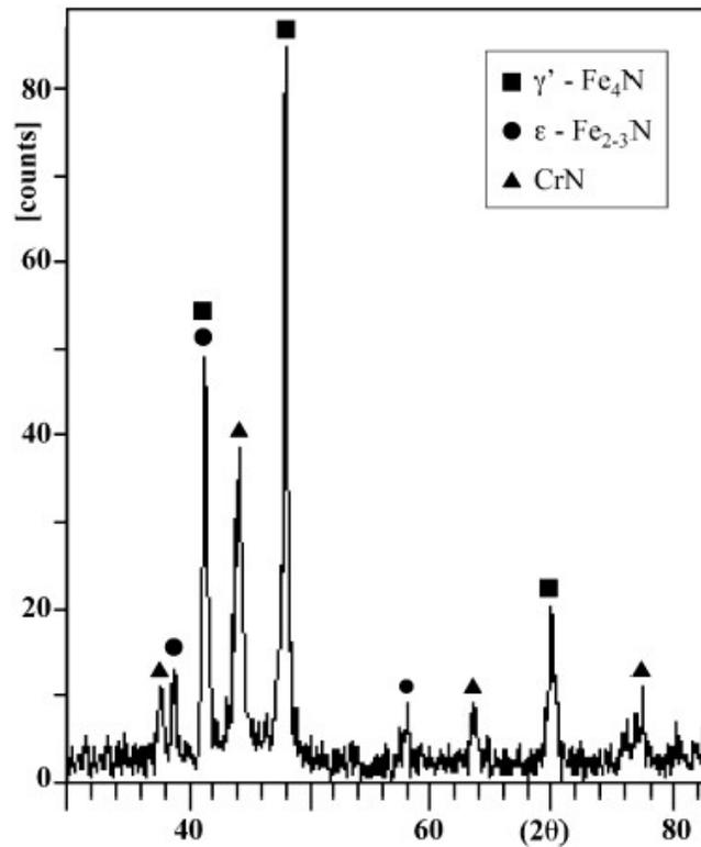
**Figure 6.** XRD diffraction pattern after nitriding at 560°C.
