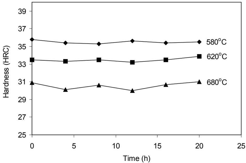
Figure 4. Aging behaviour at 520°C for samples previously double tempered at 580, 620 and 680°C.
