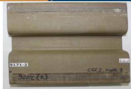
Figure 10. Aspect of the samples after hot stamping.
