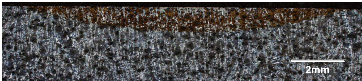
Figure 1: typical aspect of the transverse section of a laser track.
