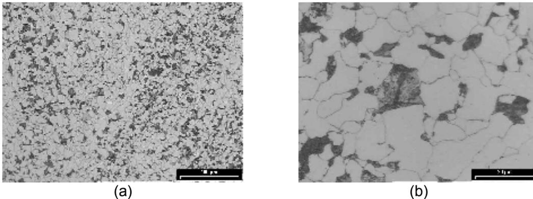
**Figure 3.** Alloy 1 Microstructure after submitted at thermal cycle with soaking temperature 1000°C por 360s. Optical Microscopy: (a) 200x, and (b) 1000x. Nital 3%.
