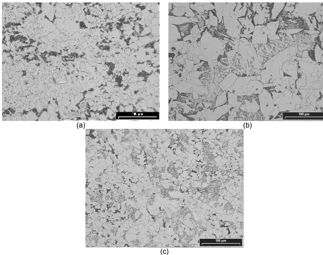
**Figure 1.** Microstructure of steels in study in as-received condition: (a) Alloy 1, (b) Alloy 2, and (c) Alloy 3. Optical Microscopy. 200x. Nital 3%.
