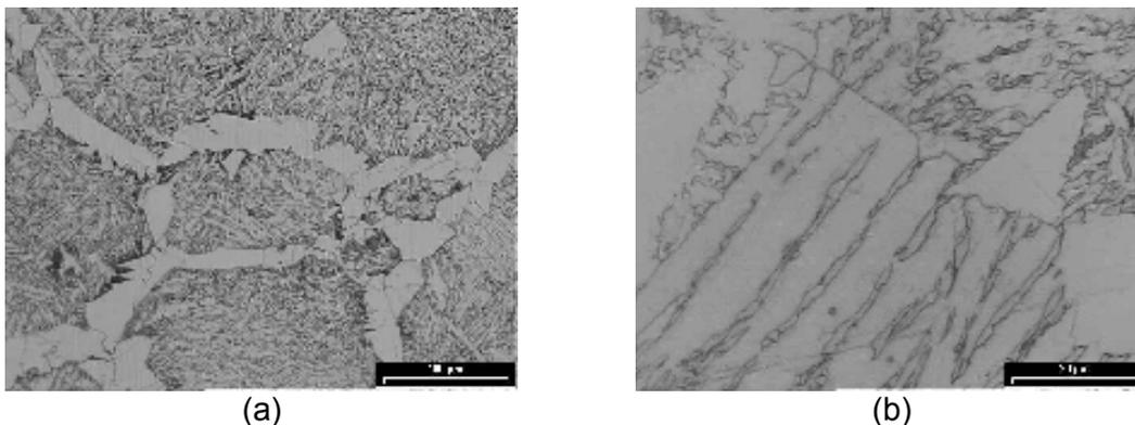
**Figure 4.** Alloy 1 Microstructure after submitted at thermal cycle with soaking temperature 1230°C por 360s. Optical Microscopy: (a) 200x, and (b) 1000x. Nital 3%.
