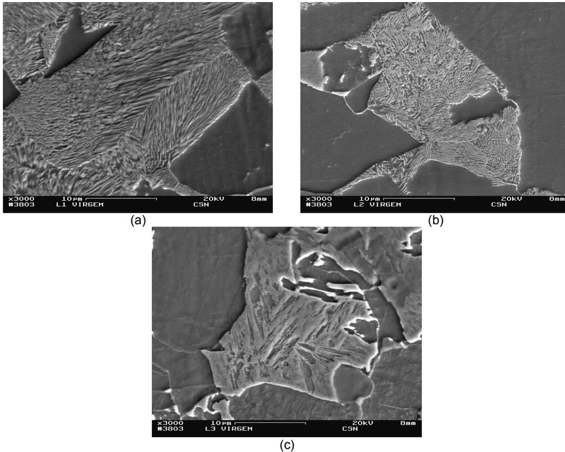
**Figure 2.** Microstructure details of steels in study in as-received condition: (a) Alloy 1, (b) Alloy 2, and (c) Alloy 3. SEM. 3000x. Nital 3%.
