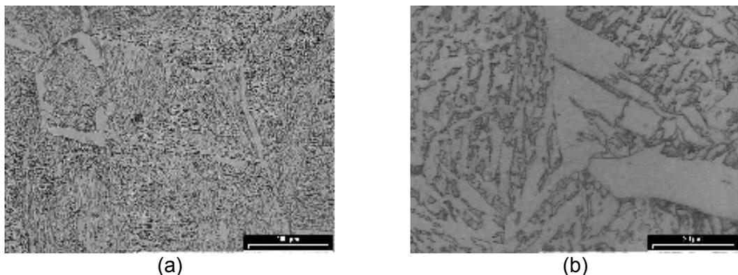
**Figure 8.** Alloy 3 Microstructure after submitted at thermal cycle with soaking temperature 1230°C por 360s. Optical Microscopy: (a) 200x, and (b) 1000x. Nital 3%.
