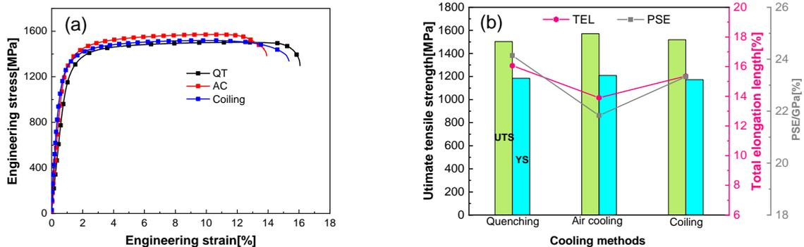
**Figure. 8** Mechanical properties obtained subject to Q&P heat treatment of austenization at 900 °C for 300s under various processing conditions:(a) Engineering stress-strain curves, (b) The yield strength (YS), ultimate tensile strength (UTS), total elongation (TEL), and product of strength (PSE) for experiment steel.
