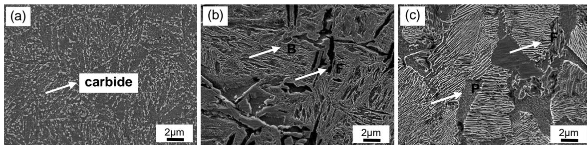
**Figure 2.** Initial microstructure of different hot rolling states (F: ferrite; B: bainite; P: pearlite), (a)—Quenching & Tempering (QT); (b)—Air Cooling (AC); (c)—Coiling.
