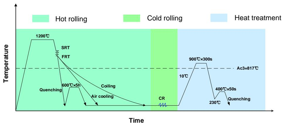
**Figure 1.** Schematic diagram of TMCP experimental steels for three different cooling procedures and Q&P heat treatment processing (SRT: Start rolling temperature; FRT: Finish rolling temperature).
