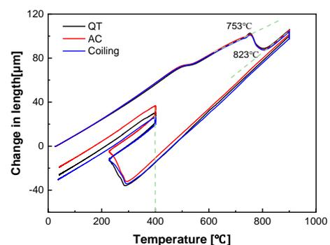
**Figure. 3** Dilatometer curve of different initial microstructures after Q&P treatment
