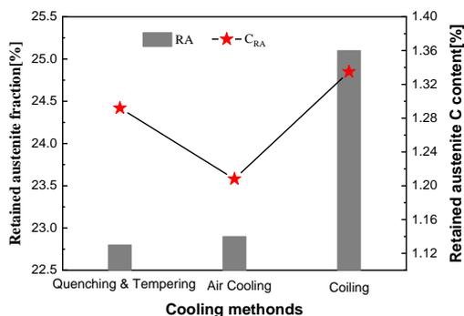
**Figure.5** Volume fraction of RA and the average carbon content in RA after cold rolling sample subjected to Q&P heat treatment
