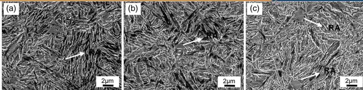
**Figure. 6** SEM diagrams of different initial structures after Q&P heat treatment (a)—Quenching & Tempering; (b)—Air Cooling; (c)—Coiling
