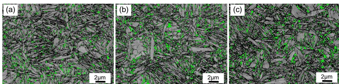
**Figure. 7** Distribution of retained austenite obtained subject to Q&P heat treatment of austenitization at 900 °C for 300s under various processing conditions. (a)—Quenching & Tempering; (b)—Air Cooling; (c)—Coiling.
