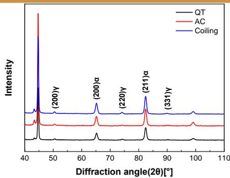
**Figure.4** X-ray diffraction patterns after cold rolling sample subjected to Q&P heat treatment
