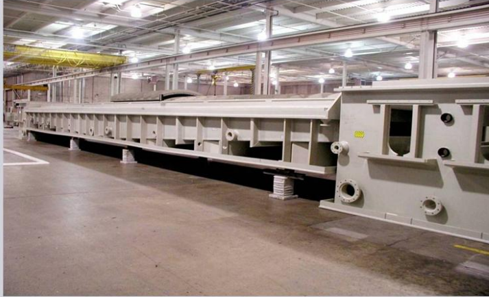
Shallow Tank with Side Injection Nozzles
