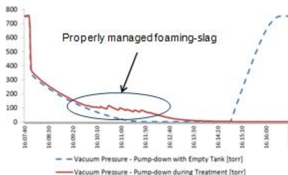
Figure 10: Comparison between VD treatment and empty-tank pump-down curves
