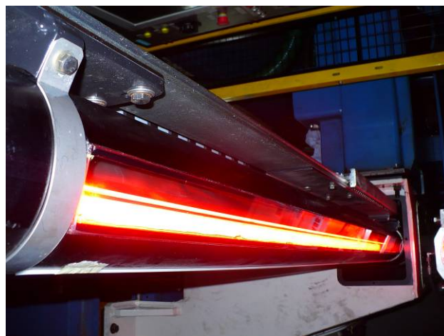
Figure 3. The lighting system is mounted on rails to be quickly extracted & checked.
