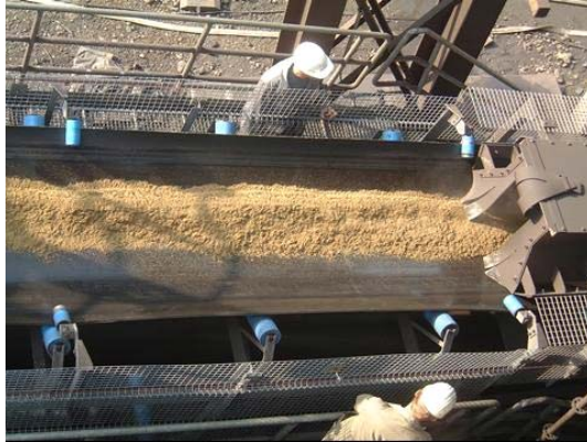
Figure 9. Granulate From The First Slag Cast As It Is Discharged From The Screw Conveyor Outlet.
