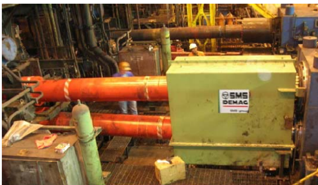
Figure 16. Complete F2 SIEFLEX® Installation June 2005 (Note - OEM Grease Lubricated Spindle in F1 can be seen in the background)
