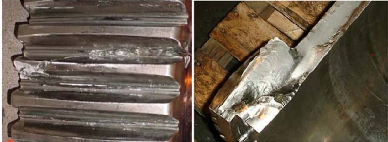
Figure 11. Gear breakage after 4 months service.
