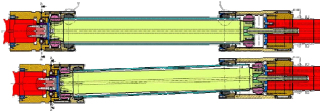
Figure 6. SIEFLEX® Cold Mill tube spindle with oil lubrication through pinion shafts
