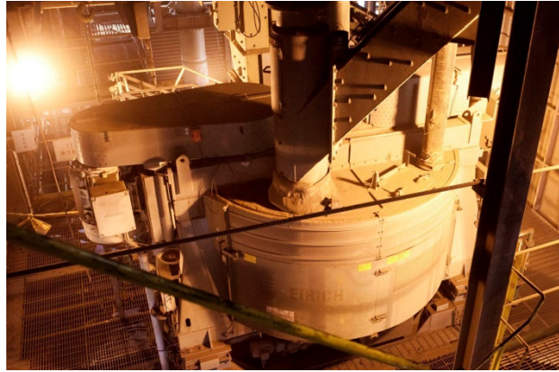
Figure 6. vertical-type intensive mixer at the sinter plant no.1, Dragon Steel Corporation.
