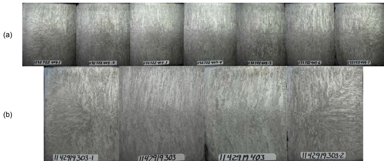
**Figure 1.** Transverse section macrographs of (a) API X65 sour slabs and; (b) API X70 non-sour slabs after macroetching revealing clean centerline conditions with no shrinkage cavities.
