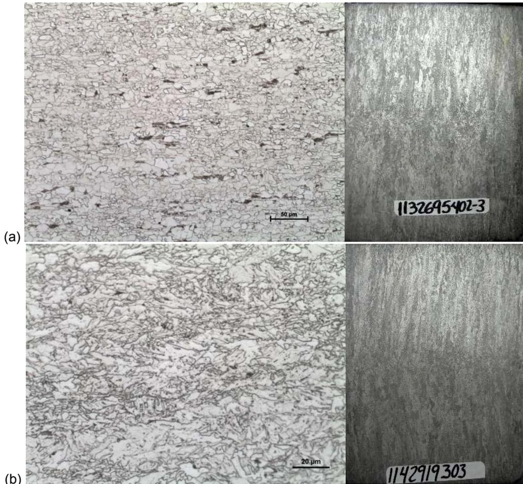
**Figure 2.** Hot rolled microstructures of (a) API X65 sour pipes; and (b) API X70 HR coil samples at mid-thickness regions revealing no banded structure of hard transformation products. The microstructures are compared with corresponding slab macrostructure after macroetching. Etched with 2% Nital.
