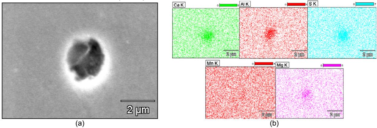
**Figure 4.** (a) Duplex Ca-aluminate and (Ca,Mn) sulfide inclusions of less than 2  $\mu\text{m}$  in sizes were observed in the steels. (b) Energy dispersive X-ray mapping indicated very low amounts of Mn present in the inclusions. Presence of Mg is also indicated and can be related to pick up from slag.
