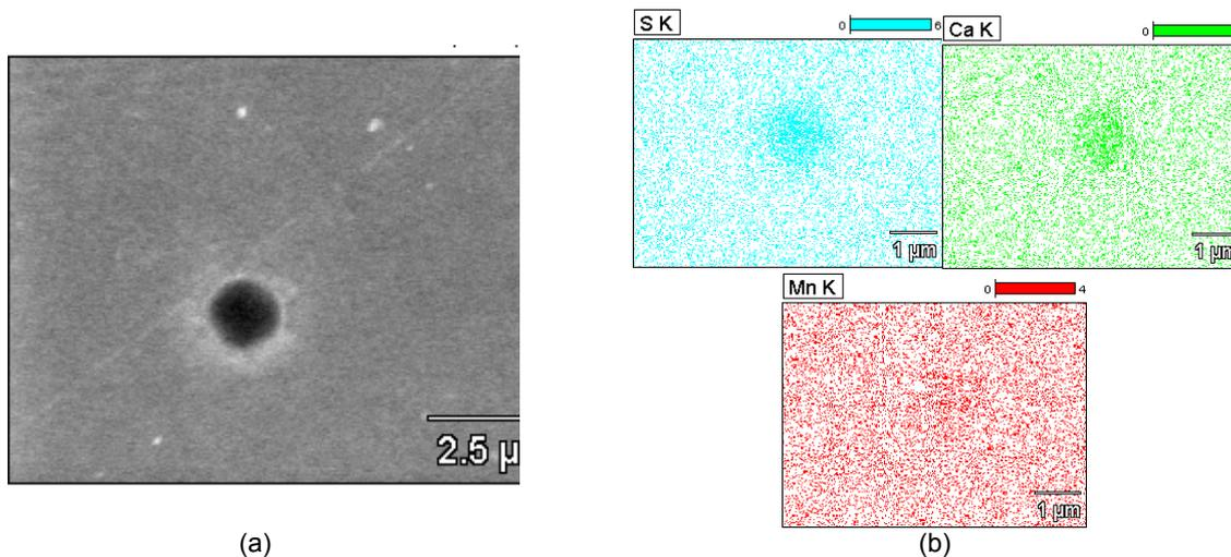
**Figure 5.** Isolated, globular, undeformed (Ca,Mn)S inclusions found in the steels with significant alloying by Ca as reflected in the X-ray mapping.
