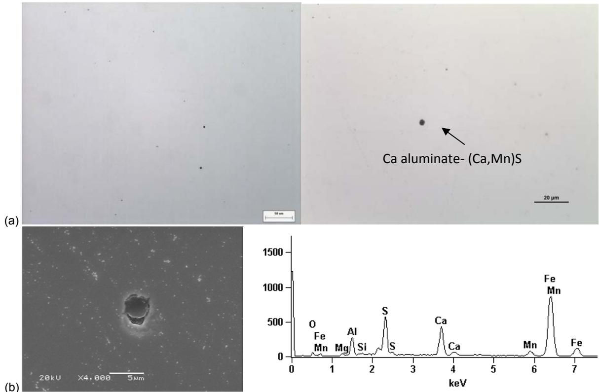
**Figure 3.** (a) Typical inclusion contents and distribution in line pipe grade heats. The inclusions are mostly oxide-sulfide conglomerate as shown in SEM-EDS microanalysis in (b) and were not deformed after hot processing.
