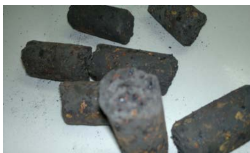
Figure 8. Brex made from HBI fines.
