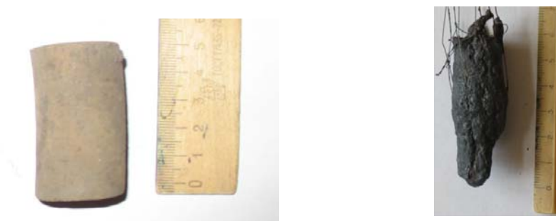
Figure 6. Sample #2-3 before and after thermal exposition at T= 1500°C.
