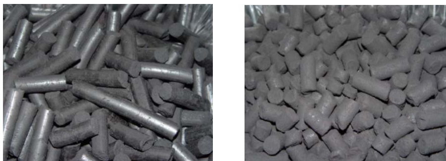
Figure 7. Coke breeze brex prior and after the tumble in rotating drum.
