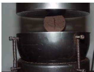
Figure 1. Position of the brex under tensile splitting test.
