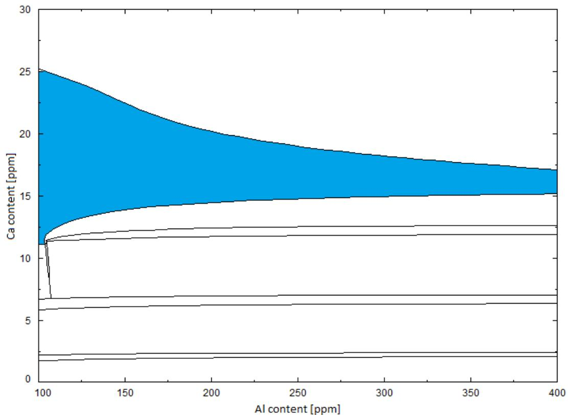
**Figure 3.** Effect of sulfur in the 'liquid window' (in blue): 50 ppm S, 20 ppm O, 1550°C
