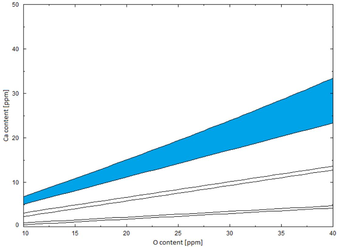
Figure 8. Profile of the 'liquid window' (in blue): 100 ppm Al, 250 ppm S, 1550°C
