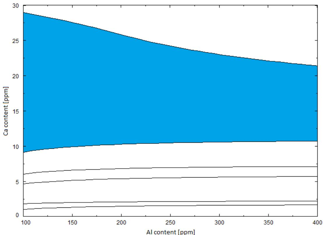
**Figure 1.** Effect of sulfur in the 'liquid window' (in blue): 50 ppm S, 20 ppm O, 1600°C
