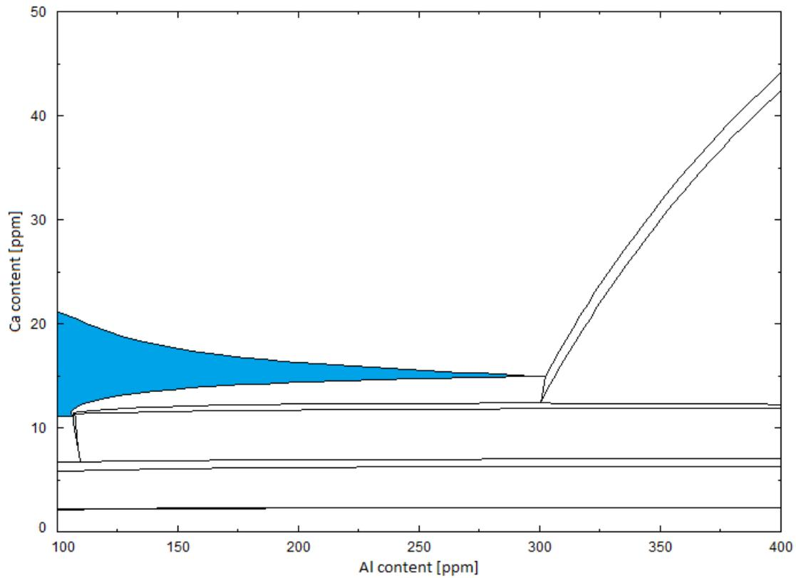
**Figure 6.** Effect of oxygen in the 'liquid window' (in blue): 20 ppm O, 100 ppm S, 1550°C
