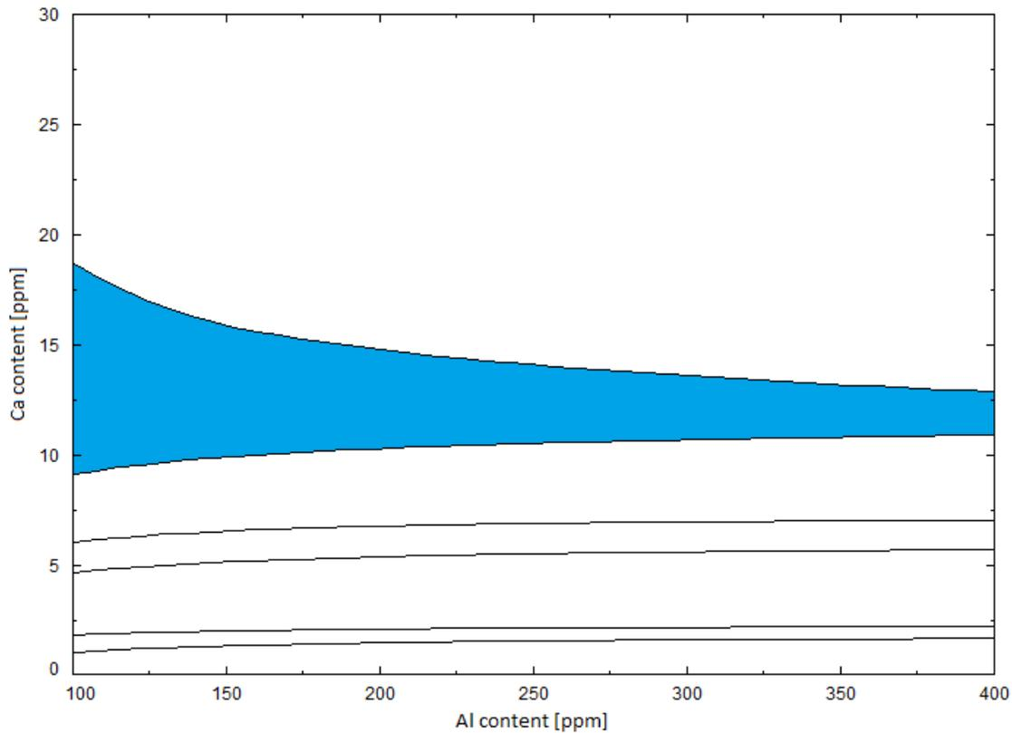
**Figure 2.** Effect of sulfur in the 'liquid window' (in blue): 250 ppm S, 20 ppm O, 1600°C
