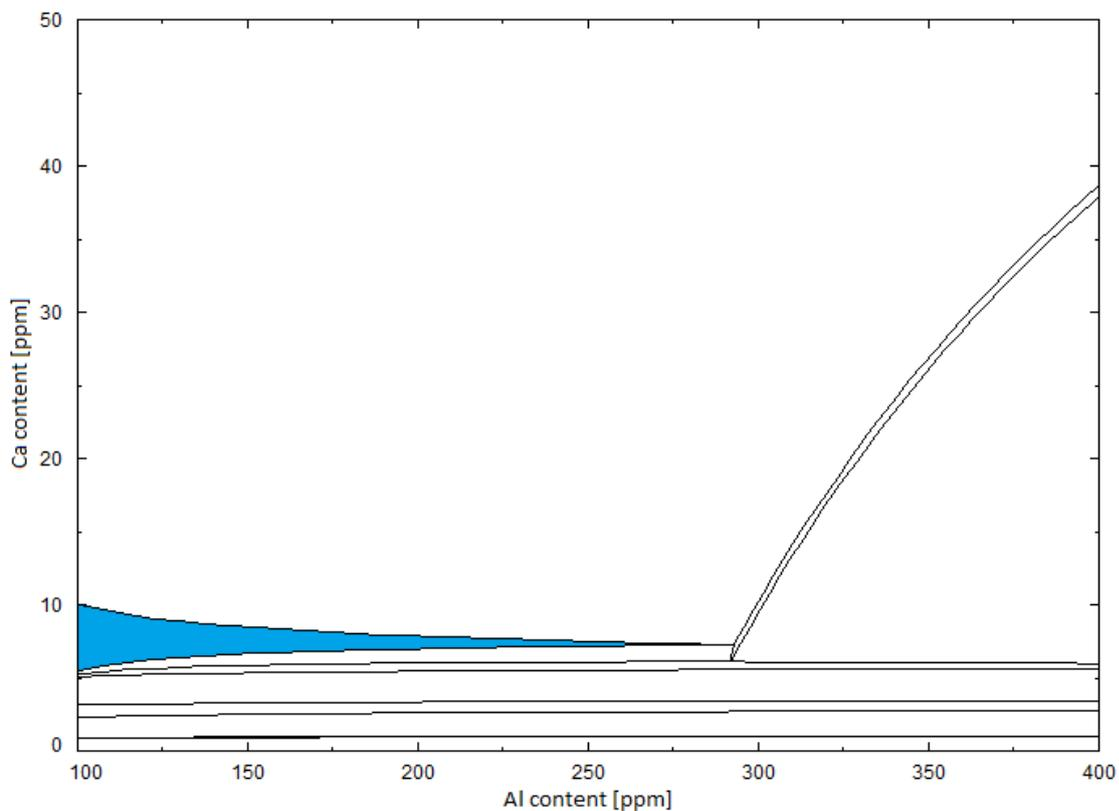
**Figure 5.** Effect of oxygen in the 'liquid window' (in blue): 10 ppm O, 100 ppm S, 1550°C
