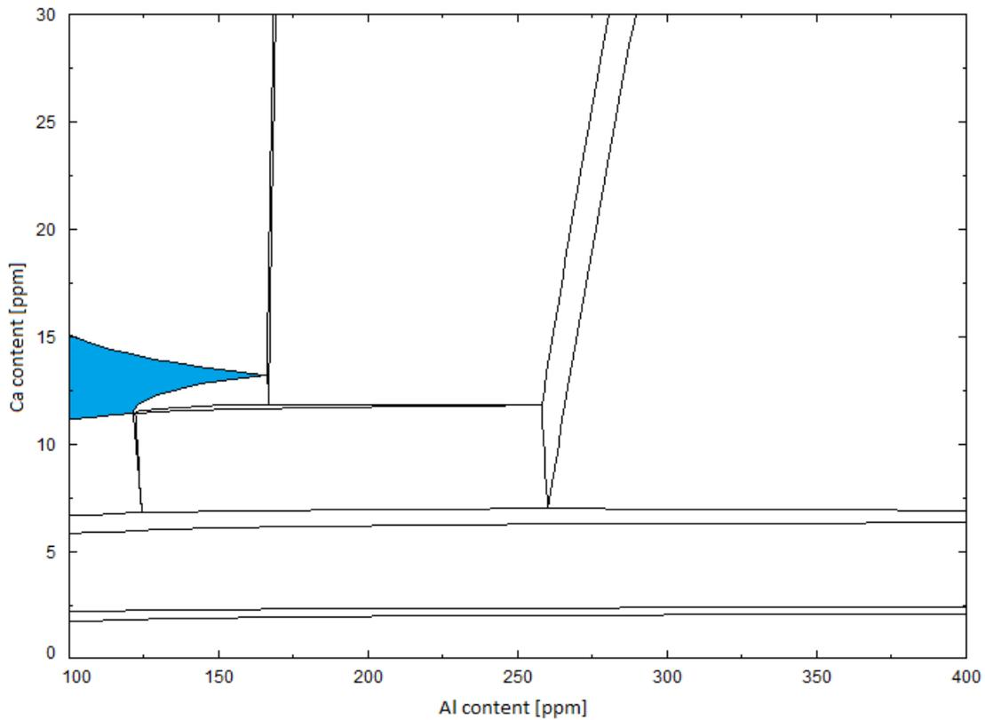
**Figure 4.** Effect of sulfur in the 'liquid window' (in blue): 250 ppm S, 20 ppm O, 1550°C
