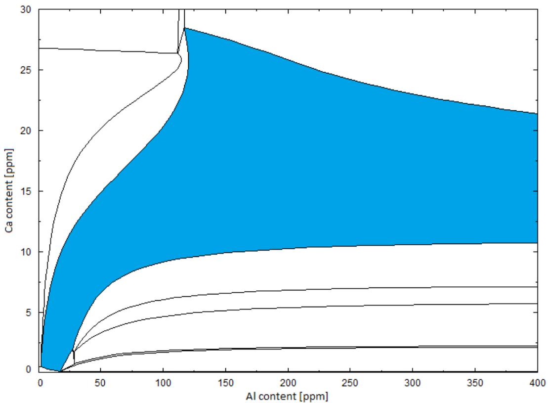
Fig.9. 'Full' view of the 'liquid window' (in blue): 20 ppm O, 250 ppm S, 1600°C
