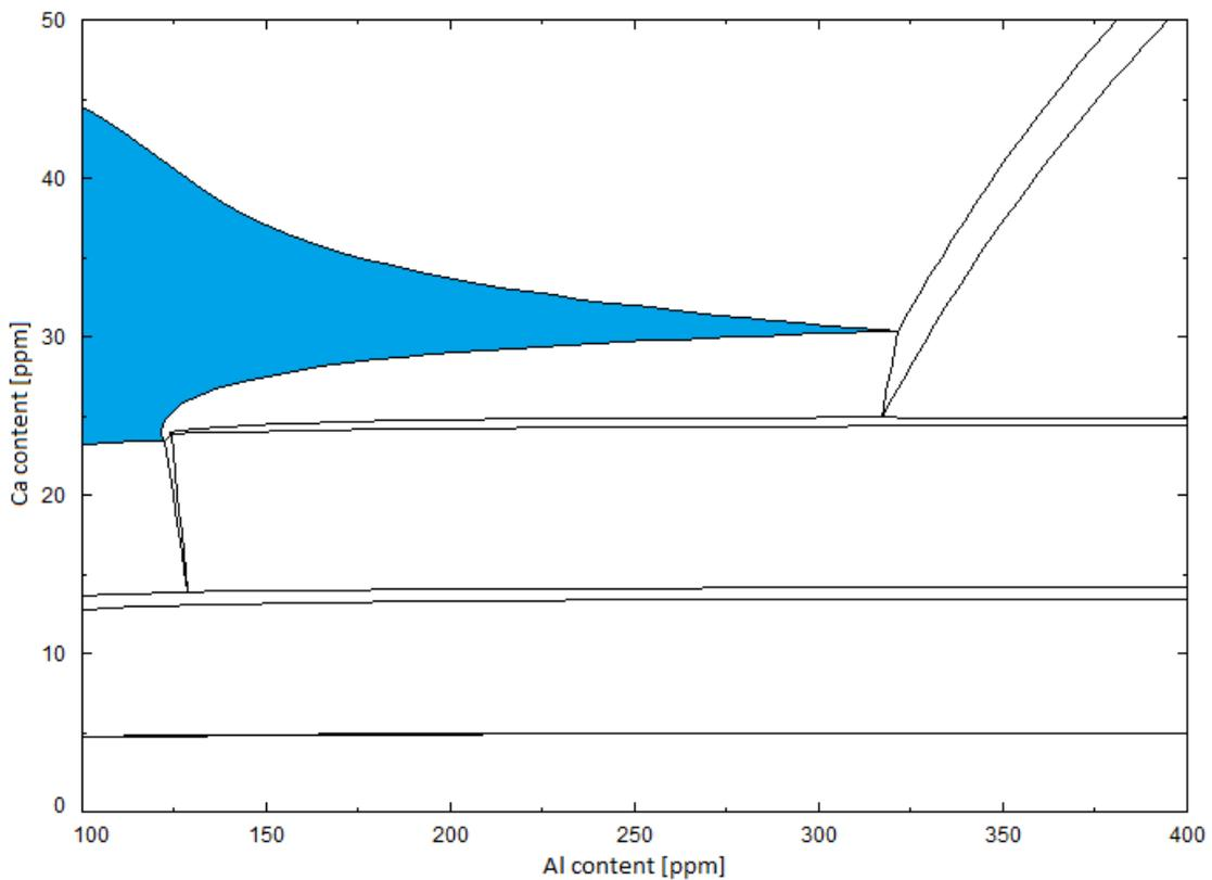
**Figure 7.** Effect of oxygen in the 'liquid window' (in blue): 40 ppm O, 100 ppm S, 1550°C
