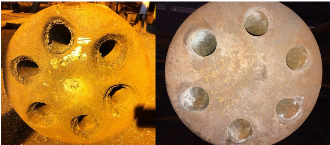
Figure 6 – Tip face photo SMS-I: a) nozzle due to over dimensioning for tip, b) Slagless Clean Up after 523 heats.
