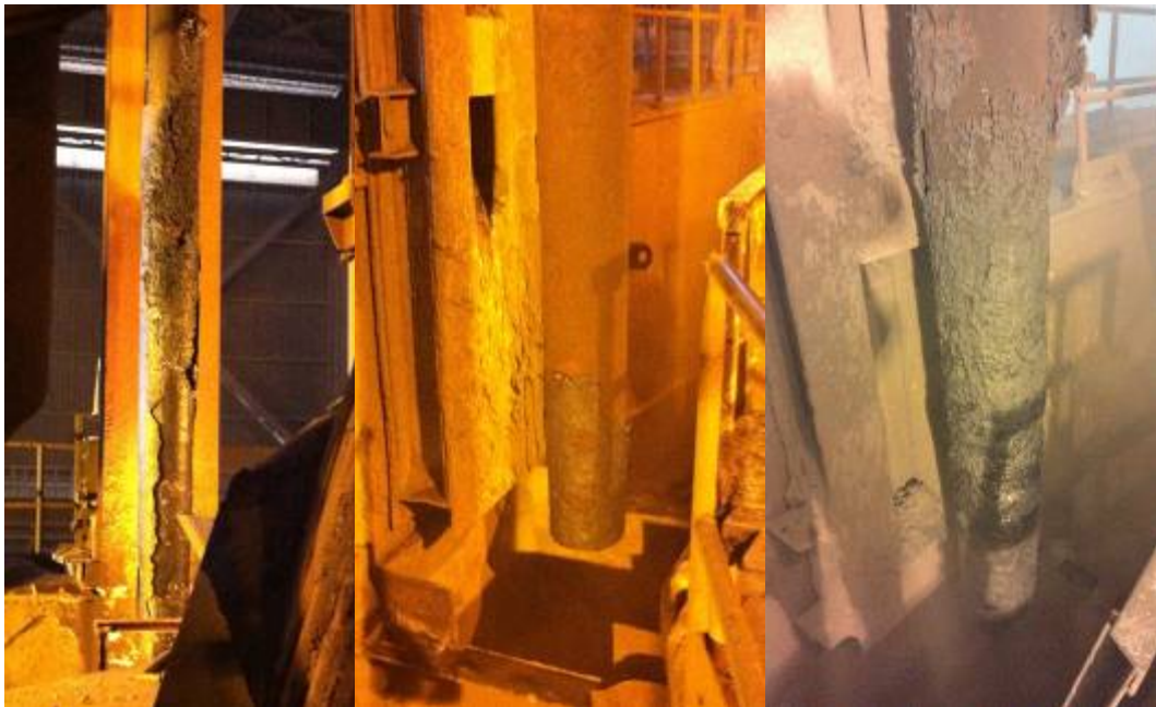
Figure 2 – Kinds of jam's formation: a) slag, b) metallic and c) mixer.
