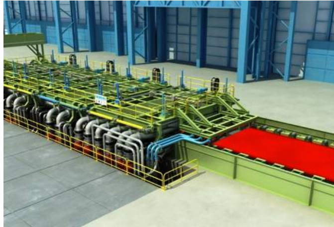
Figure 9. The MULPIC® Cooling System.
