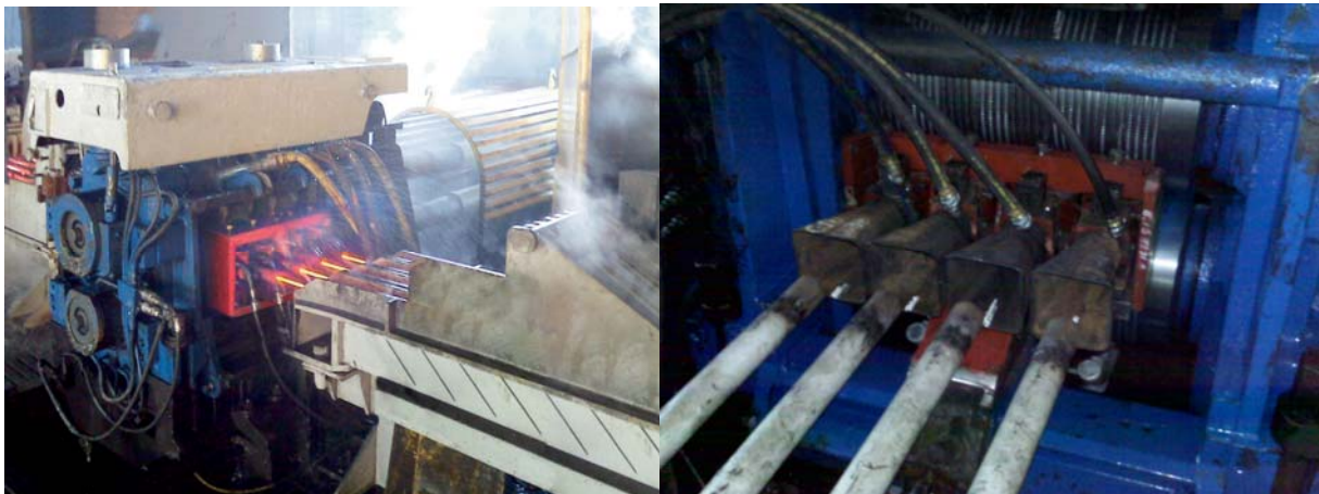
Figure 5: Exit twisting guide RTC and entry guide SR type.
