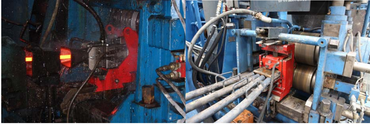
Figure 4: Entry guide MDR and slitting guide MSL45.
