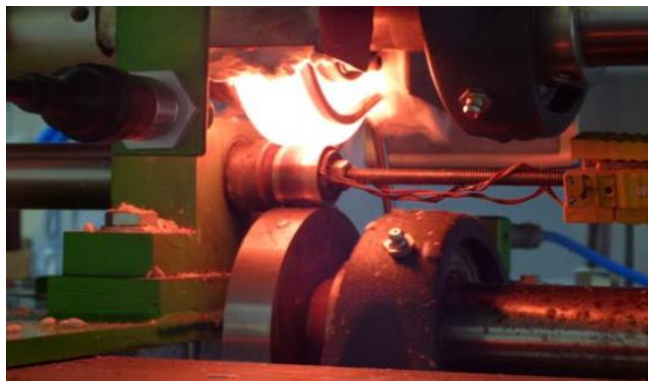
Figure 3. The Hot Rolling Simulator (3 discs configuration).
