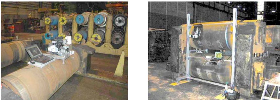
Figure 7. On-site microscopy with a portable microscope a) microscope on the roll; b) microscope fixed vertically.
