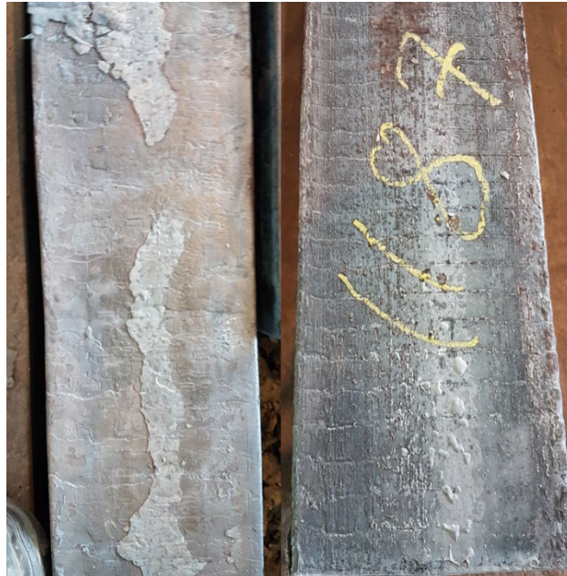
Figure 10: Comparison of a regular billet cast with opened stream (strand 1 – left) and a billet cast with CNC Shroud with flux powder (strand 6 – right).
