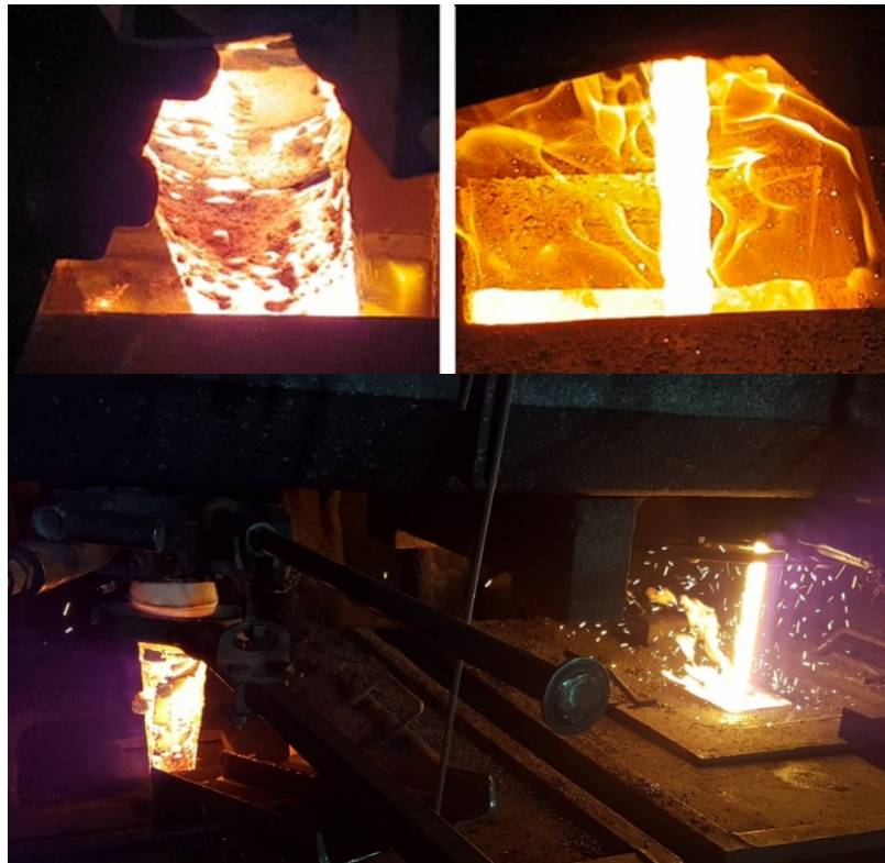
Figure 7: Casting from tundish to mold with open stream (right-hand side) and Shrouded stream (left-hand side).
