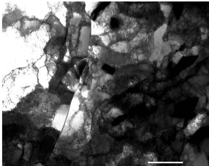
Fig.5 - TEM micrograph: Several grains containing a random sub-grain structure with some cellular structure inside them and some identified precipitates in the annealed 6063 Al alloy who was cold drawn (1 step, 20%) and cold deformed on torsion (20 cycles, 2.8%).  $Z \approx (011)$ ; (Bar =  $5\mu\text{m}$ )
