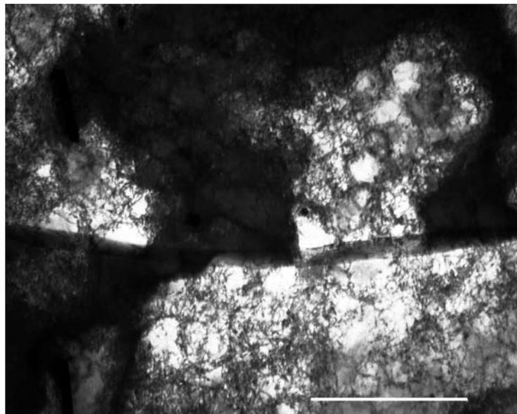
Fig.3 - TEM micrograph: Fine and regular cell structure and presence of same identified precipitates in the annealed 6063 Al alloy who was cold deformed in torsion (2.8%) and finally cold deformed on tensile test.  $Z \approx (013)$ ; (Bar =  $5\mu\text{m}$ )
