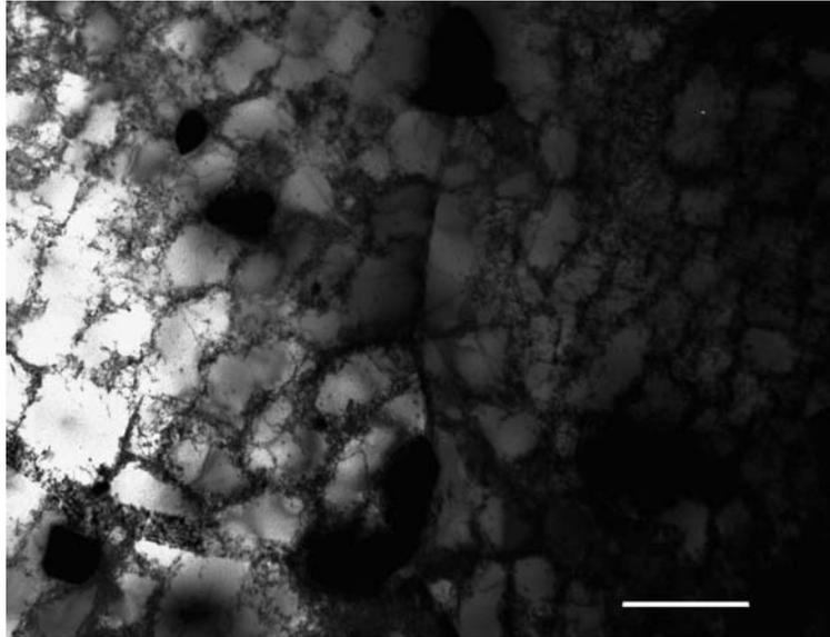
Fig.2 - TEM micrograph: An intense and regular cell structure in the three observed grains in the annealed 6063 Al alloy that was cold deformed in torsion for 20 cycles, 2.8% strain per cycle.  $Z \approx (011)$ ; (Bar =  $5\mu\text{m}$ )
