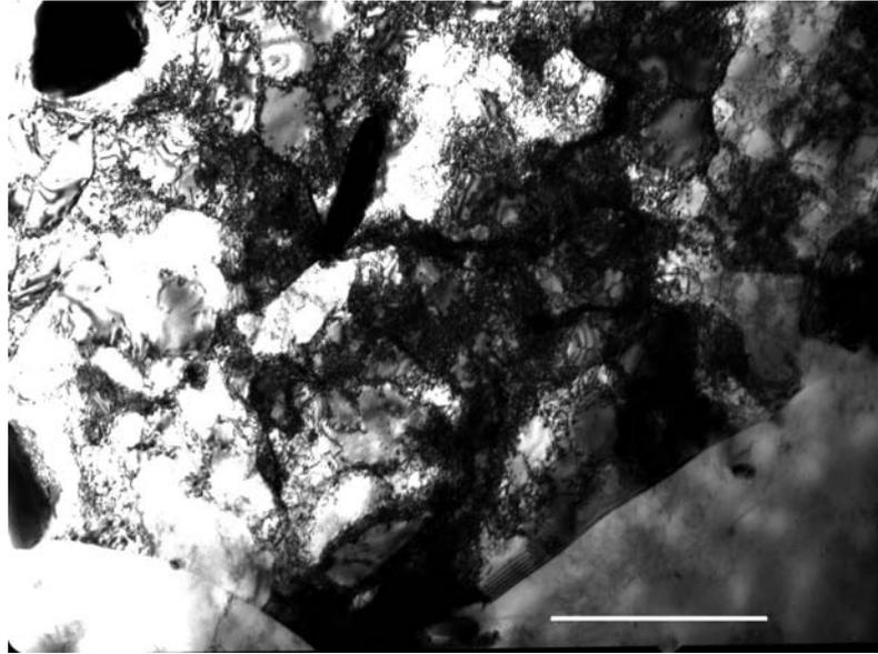
Fig.6 - TEM micrograph: Fine sub-grains, dislocation tangles near each sub-boundary and some types of precipitates in the annealed 6063 aluminum alloy who was cold drawn (1 step, 20%) and cold deformed on tensile test.  $Z \approx (011)$ ; (bar = 5 $\mu$ m)
