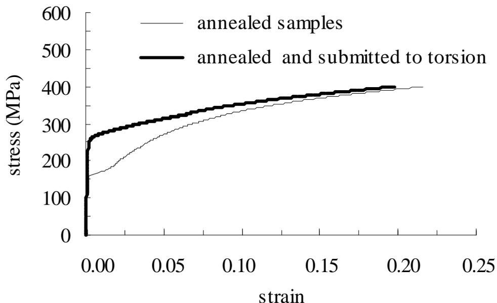
Fig.1. Stress x strain curves obtained in 6063 aluminum alloy (annealed; annealed and torsion process)
