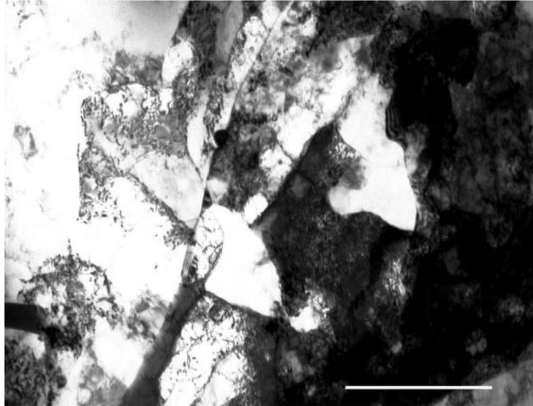
Fig.4 - TEM micrograph: Sub-grains structure and a dislocation network inside the grains in the annealed 6063 Al alloy who was cold drawn (2 steps, 20% each one).  $Z \approx (011)$ ; (Bar =  $5\mu\text{m}$ )
