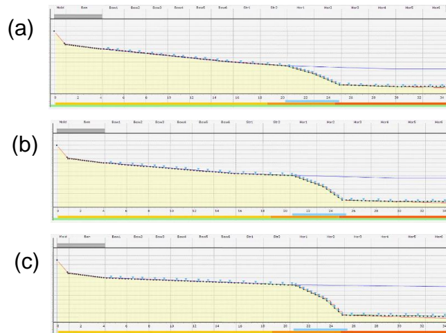
Figure 15. Gap profiles shown in the Level 2 HMI during the trials: (a) Standard soft reduction practice using Smart Segments, SRD practices with increased reduction 150% (b) and 200% (c) using SRD Segments.
