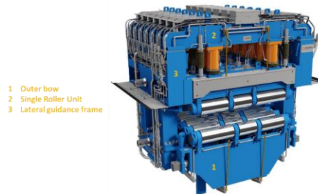
Figure 9. Assembly of the SRD Segment.
