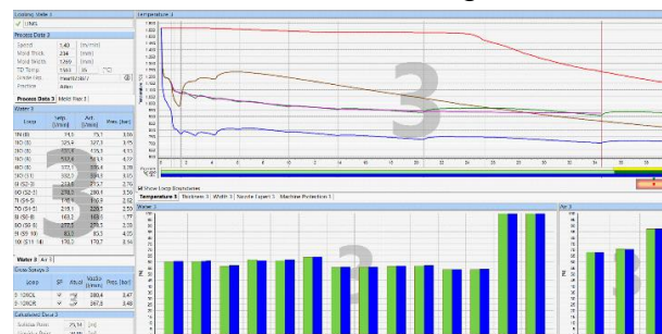
Figure 5. Dynacs 3D implemented in Level 2 HMI.
