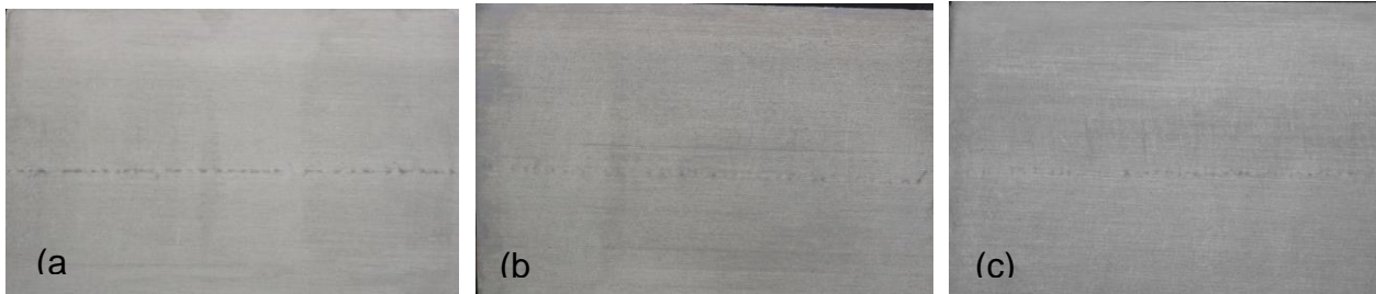
Figure 18. Macro etches of Trial 3. Application of standard soft reduction practice using conventional Smart Segments (a), increased soft reduction (125%) using SRD Segments (b) and increased soft reduction (150%) using SRD Segments (c).
