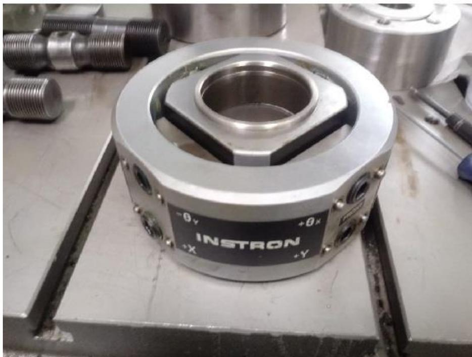
Figura 9. Instron Alignment Fixture Model 8000-073 (photo and schematic [5]).
