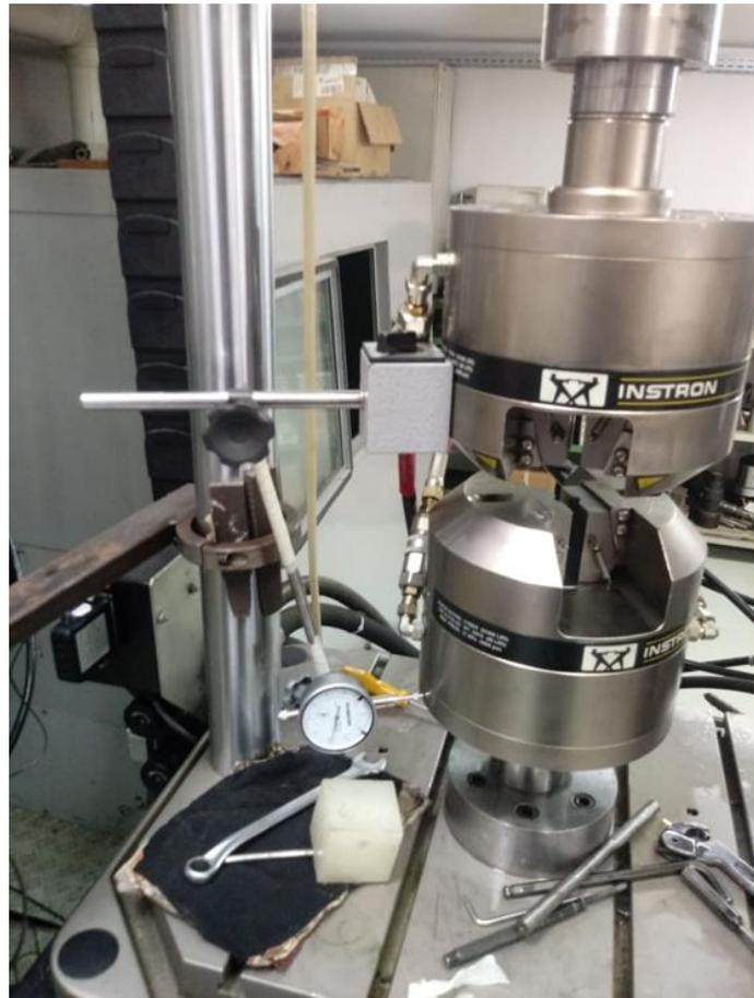
**Figure 6.** Example of an assembly for the Dial Indicator Method.
