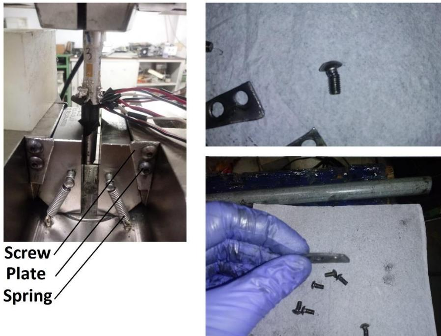
**Figure 2.** Bending of plates and shearing of screws, caused by the use of a misaligned system. Moreover, if the specimen's buckles, the resulting misalignment increases the chance of a grip to rotate and, therefore, the hydraulic piston column to bend. If subjected to enough bending moment, the column deformation can be irreversible, causing machine malfunction (Figure 3).
