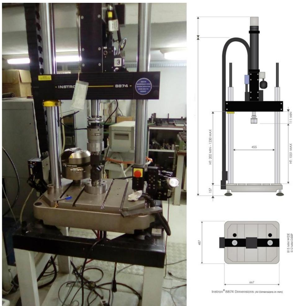
**Figure 1.** INSTRON 8874 Biaxial servohydraulic fatigue testing system (photo and schematic [1])
