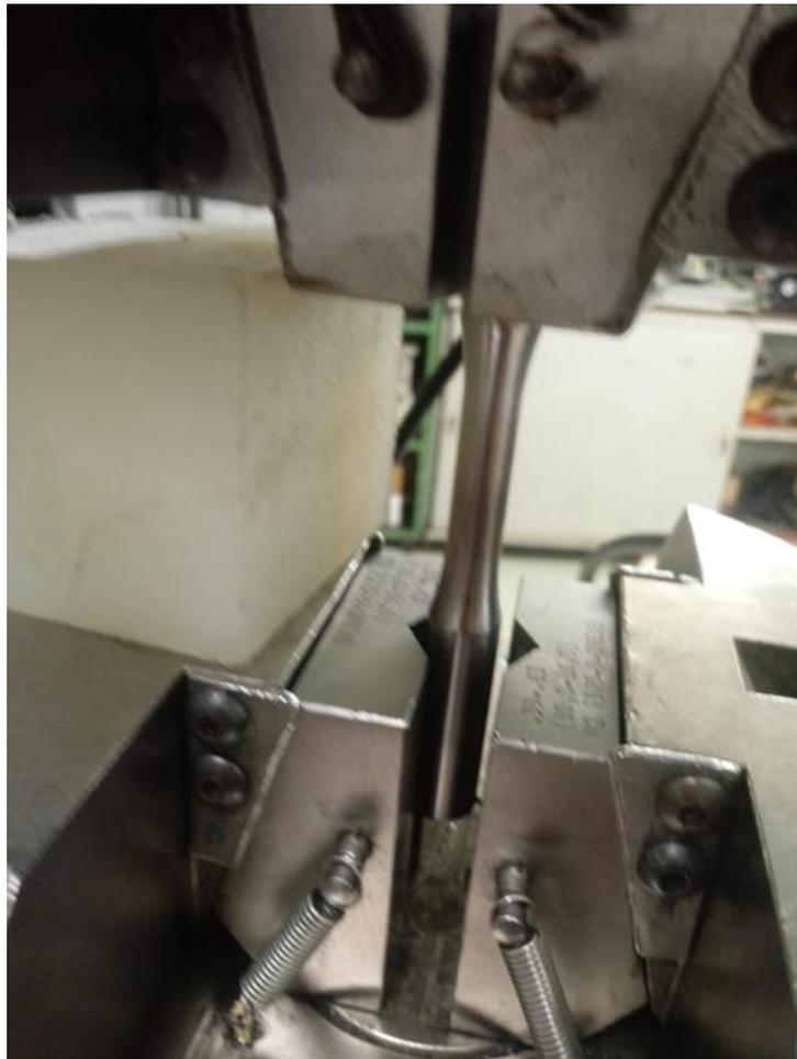
**Figure 5.** Example of a considerably misaligned assembly. The specimen should be within the same distance from each jaw face.
