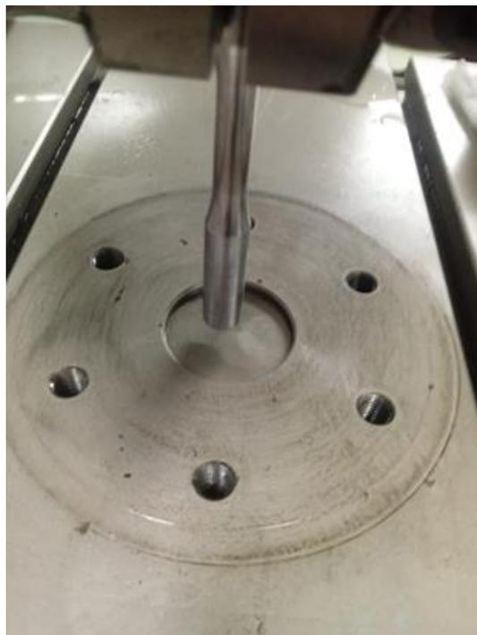
**Figure 3.** Misalignment caused by a bent hydraulic piston column. The specimen should be pointing towards the center of this circle.
