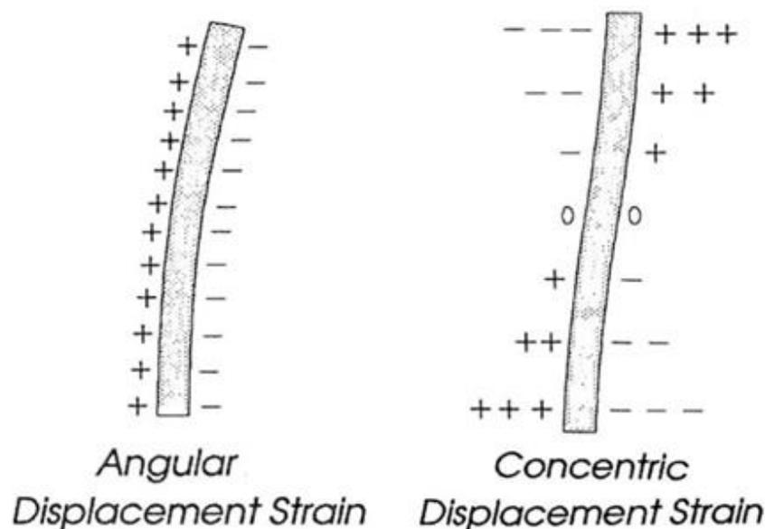
**Figure 10.** Types of strain displacement on the specimen [5].
