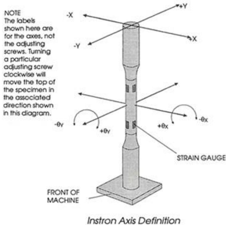
**Figura 11.** Schematic of the strain gauge configuration for this reading [5].
