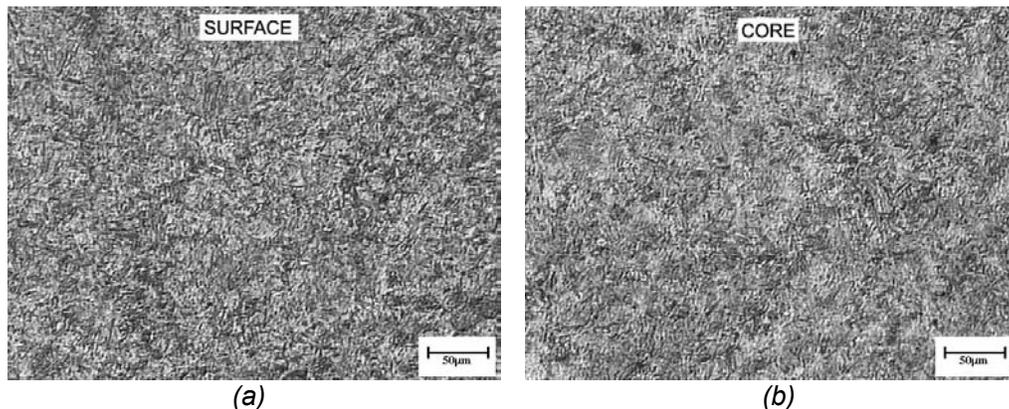
Figure 8. Microstructure of 4140 steel, quenched in water (30°C). a) Surface sample, b) core sample. They show martensitic microstructure.
