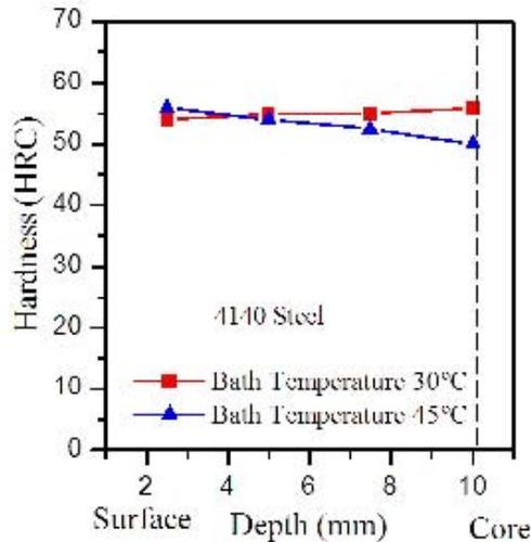
Figure 7. Hardness profile of 4140 steel, quenched in water, with different bath temperatures.
