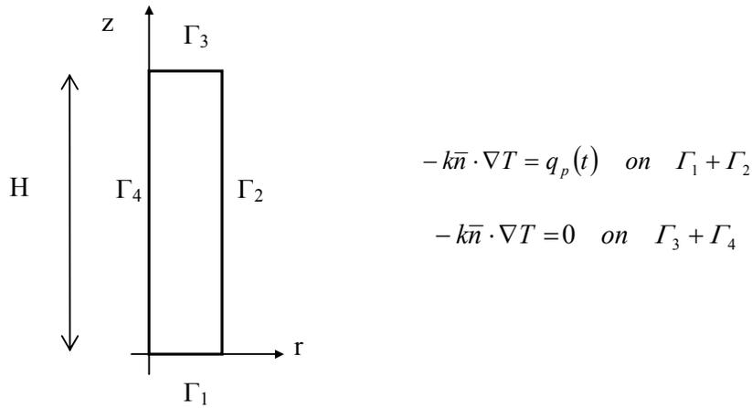
**Figure 11.** Calculation domain and applied boundary conditions.
