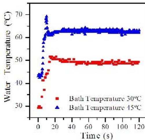
Figure 6. The effect of the water temperature during cooling of 4140 steel.
