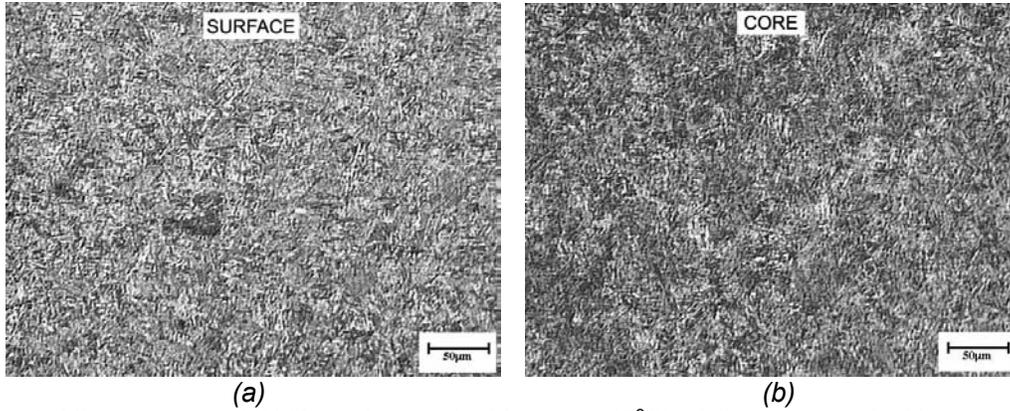
**Figure 9.** Microstructure of 4140 steel, quenched in water (45°C). a) Surface sample, b) core sample. They show martensitic microstructure.
