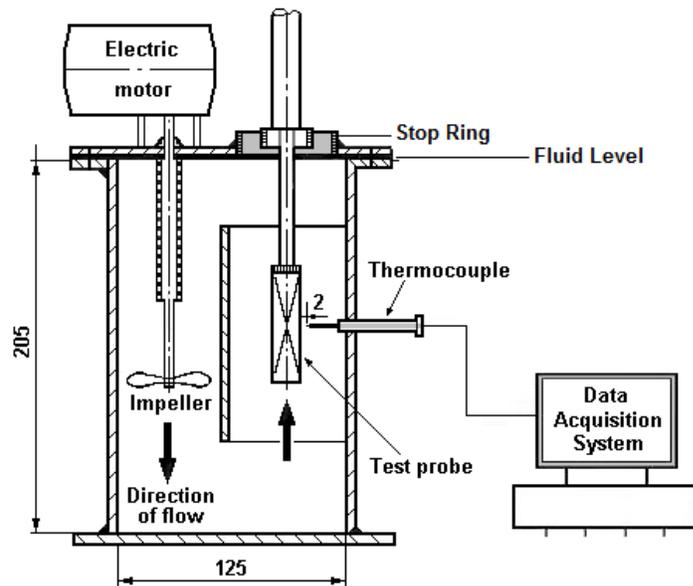
**Figure 2.** Schematic illustration of the laboratory quenching and data acquisition system.
