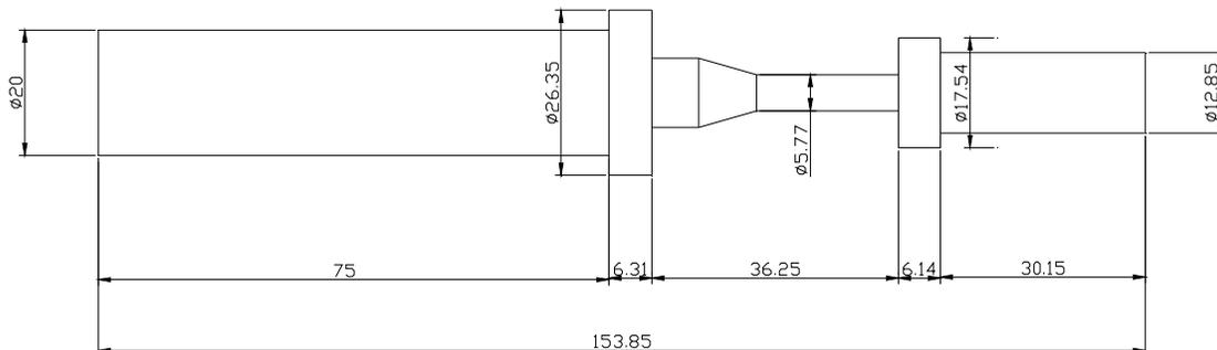
**Figure 4.** Schematic illustration of the dimensions of the test probe and the handle shown in Figure 3.
