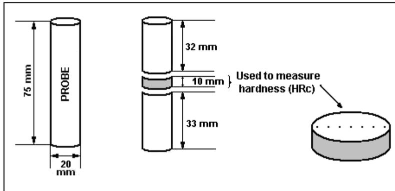
**Figure 5.** Bar sectioned used to measurement hardness (HRC).
