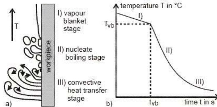
**Figure 1.** a) Different cooling stages on a workpiece surface (increasing workpiece surface temperature from bottom to top); b) Variation of the surface temperature during quenching.
