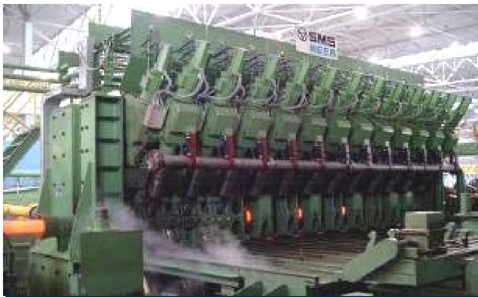
Figure 12: SRM - Stretch Reducing Mill type 310 A with 24 stand positions.
