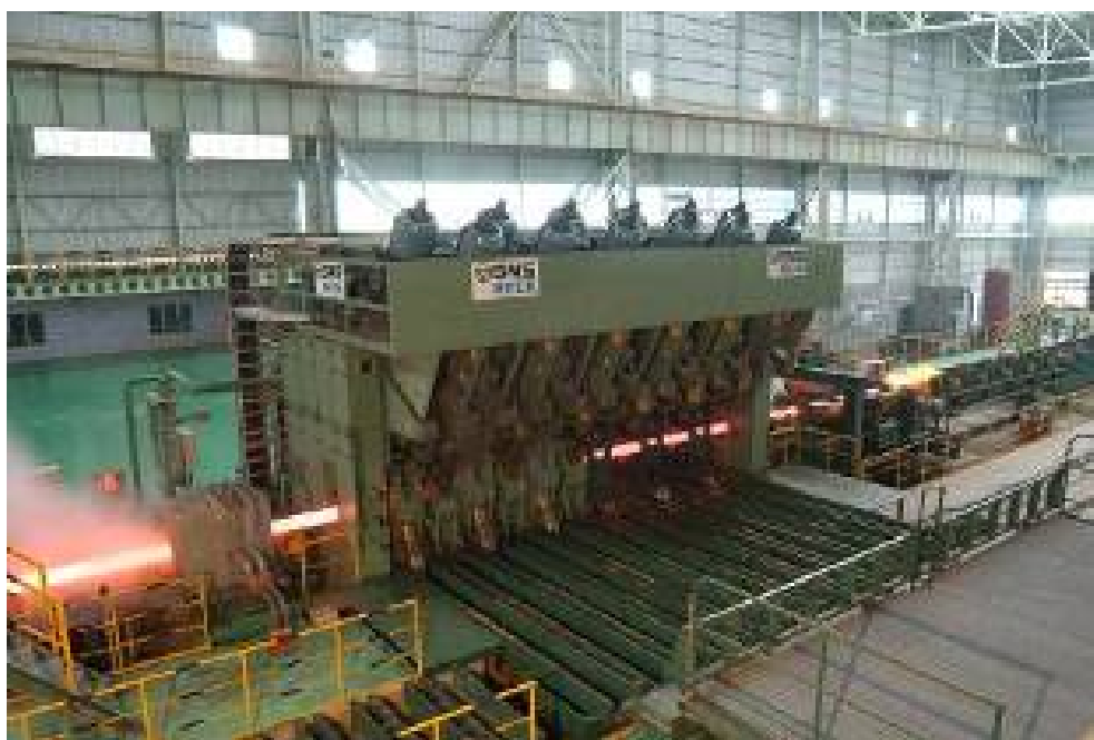
Figure 13: Sizing Mill type 670 A with 12 stand positions, single roll drive system – one motor per roll.
