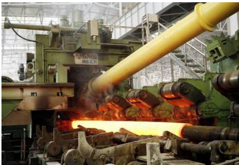
Figure 5: Largest piercing mill in operation in a 18" PQF mill at TPCO / China.
