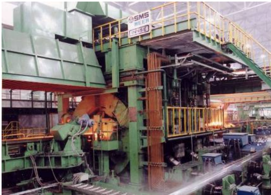
Figure 6: First 6 5/8" PQF® mill in operation at TPCO / China.
