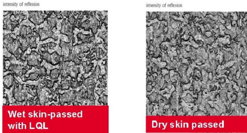
Figure 14. Comparison of the strip surface quality with and without low quantity lubrication.
