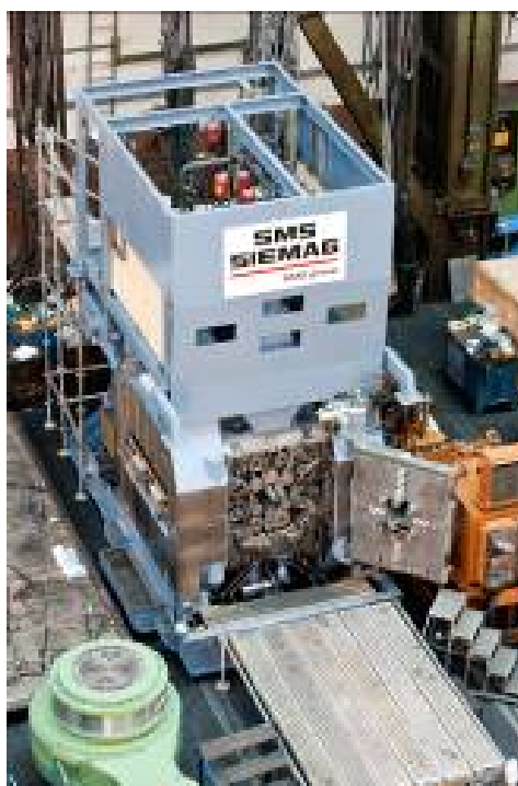
Figure 10. MB 22-B52" mill for Hunan Xiangtuo Goldsky Titanium Metal Company, carried out in all-in-one modular design, manufactured, pre-assembled in the Hilchenbach workshops of SMS Siemag.
