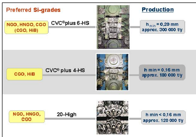
Figure 7. Mill concepts for silicon steel rolling by SMS Siemag.
