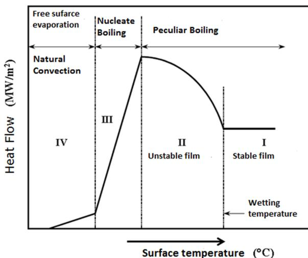
**Figure 16.** Schematic representation of the boiling curve of water on the surface of a heated plate<sup>(15)</sup>
