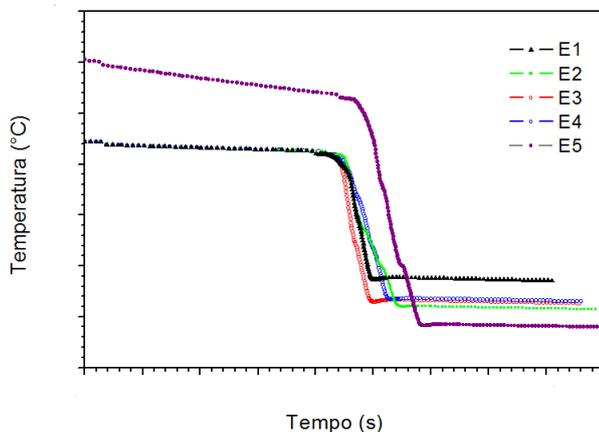
**Figure 5.** Cooling curves in different strategies of water flow in the zones
