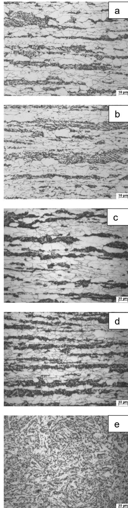
**Figure 7.** Microstructure seen in the optical microscope with magnification of 1000X to  $\frac{1}{4}$  of the thickness. a) E1 strategy; b) E2 strategy; c) E3 strategy; d) E4 strategy; e) E5 strategy
