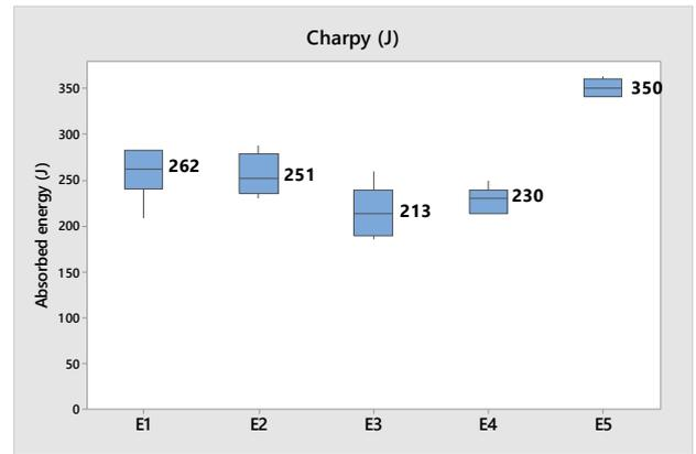
Figure 13. Absorbed energy in Charpy CVN tests in each strategy.
