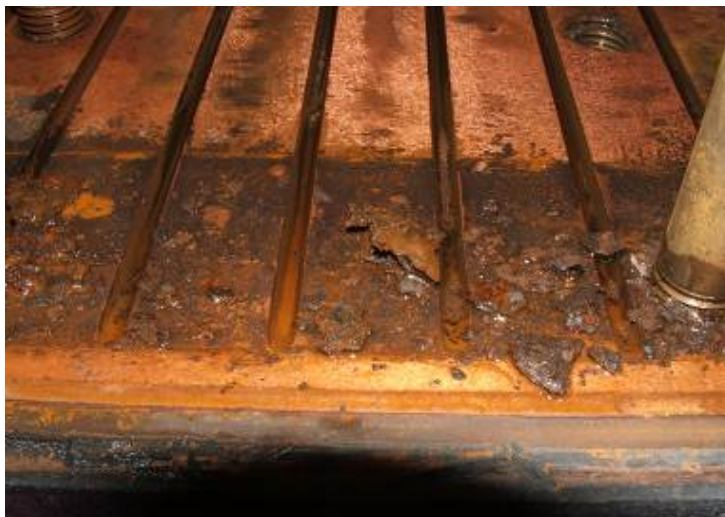
Figure 12. Scale found trapped against the slots across the bottom of a copper.
