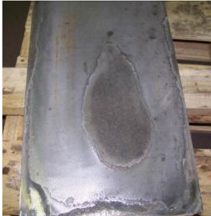
Figure 4. Nickel plated copper with typical wear.
