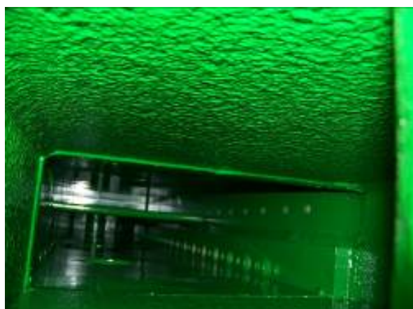
Figure 16. Mold frame after blasting and powder coating.
