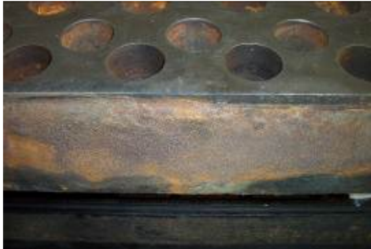
Figure 10. Eroded broad face back-up plate.
