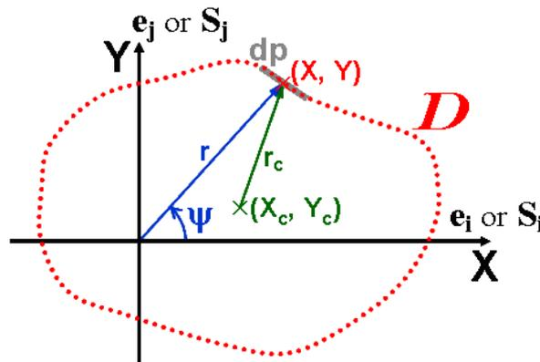
**Figure 2.** Load history path, assumed as a homogeneous wire with unit mass in the deviatoric 2D space.
