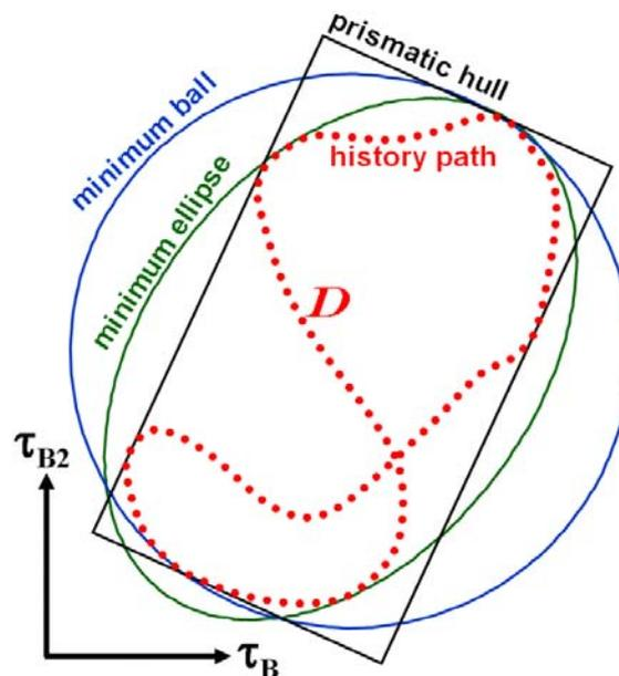
**Figure 1.** Periodic (or single) stress history path  $D$  in a  $\tau_B \times \tau_{B2}$  diagram, enclosed in surfaces such as circles (balls), ellipses and rectangular prisms.
