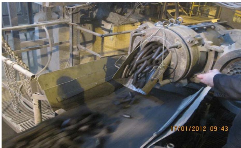
Figure 1. Industrial brex production by Steele Extruder 25 at Suraj Products Ltd.
