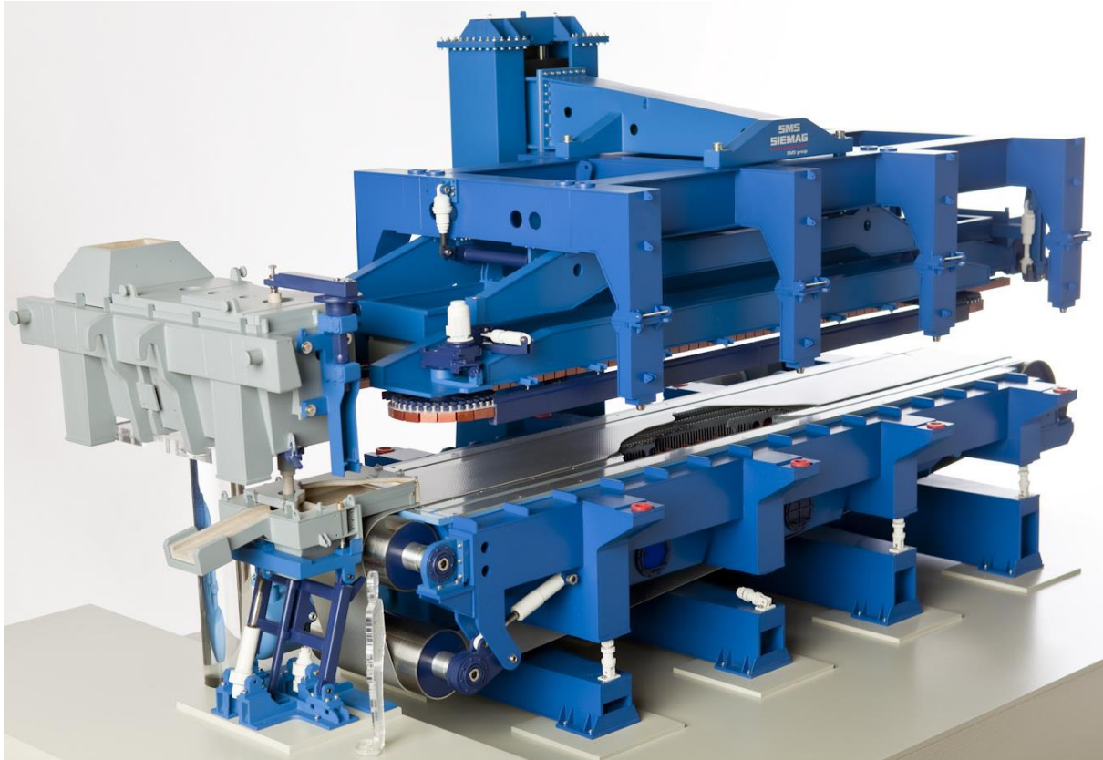
Figure 3: Tundish, feeding system and BCT® caster with lifted top frame
