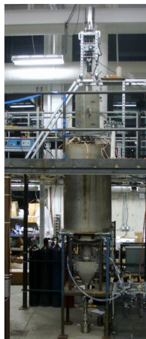
Figure 2. Utah Laboratory flash reactor: (a) schematic diagram; (b) photograph.
