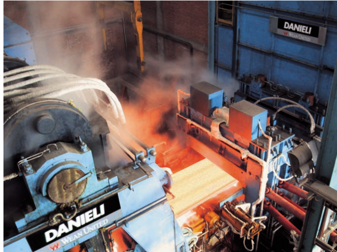
Figure 1. Casting of 85-mm-thick slabs at Tangshan fTSR complex, PR of China. The caster features the latest Danieli Thin slab Casting Technology such as H2 Funnel Mould and Dynamic Soft Reduction Control.
