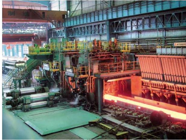
Figure 4. Strip exiting the Danieli two-stand roughing mill: the line ensures the production of ultra-thin strip down to 0.8 mm.
