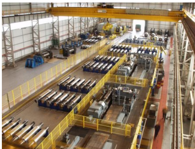
Figure 2: Example for an automated roll shop [4]
