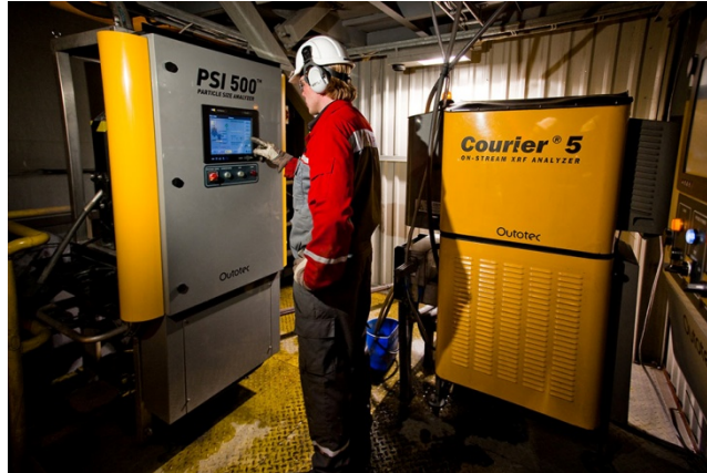
Figure 3 Laser scatter on-line particle size analyzer and XRF on-line slurry analyzer.
