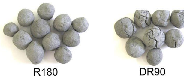
Figure 4. Typical aspect of reduced pellets after final reduction under the R180 and the DR90 conditions
