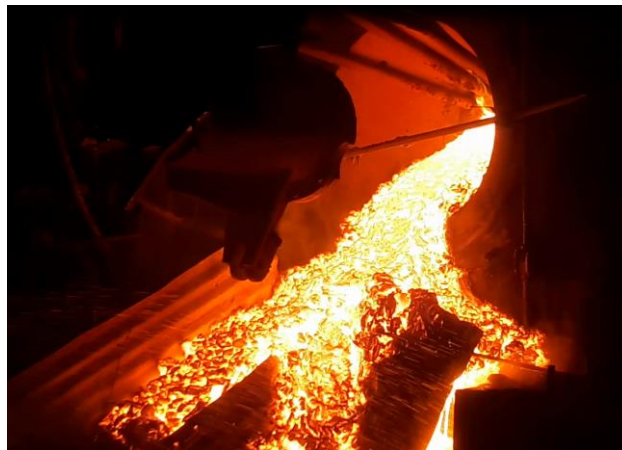
Figure 4. Slag from tuyeres.
