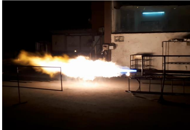
Figure 5. Test firing of lancing equipment.
