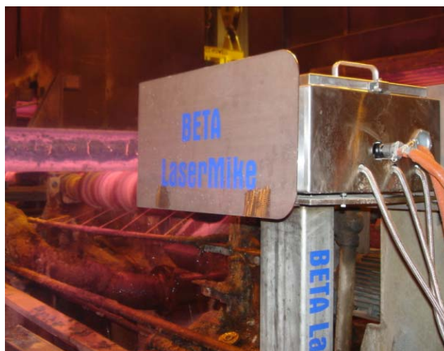
Figure 4. Side-mounted gauge on a slab caster.
