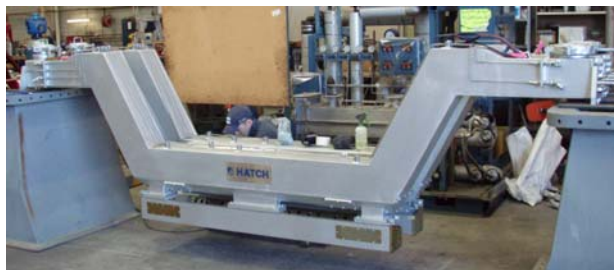
Figure 6 - Achieva Flotation Stabiliser built into the Achieva CE Air Knife Beams
