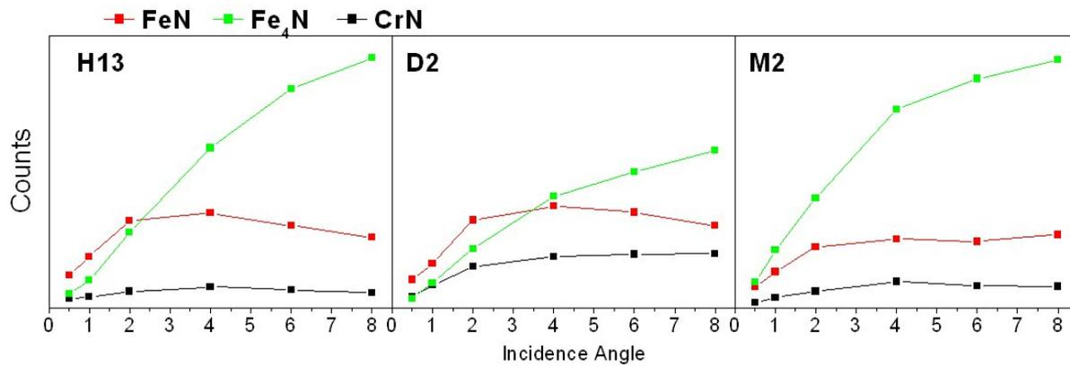
**Figure 5.** Peak height evolution of Fe<sub>4</sub>N, FeN, and CrN with incidence angle in the GIXRD of AISI H13, AISI D2 and AISI M2 (same ordinate scale).
