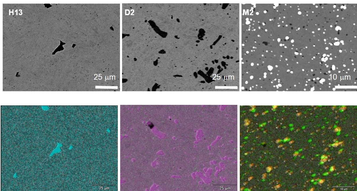
**Figure 2.** (a) BEI micrographs from AISI H13, AISI D2 and AISI M2 steels. (b) Characteristic x-ray element maps identifying some of the elements that form the inclusions (Si cyan) and carbides (V green, Cr magenta, Mo yellow, W red) on the respective images above.
