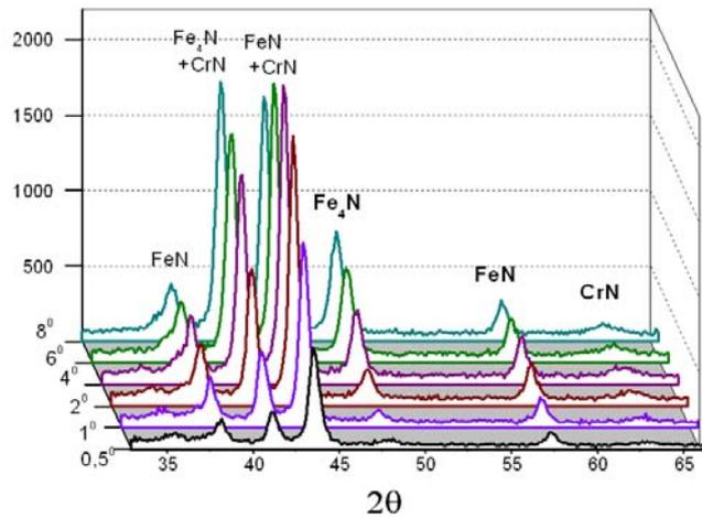
**Figure 4.** GIXRD with different incidence angles of AISI H13 after nitriding at 400°C.
