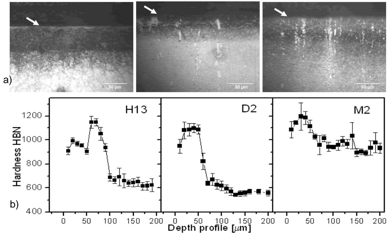
**Figure 6.** a) Cross section optical micrographs (surfaces indicated with white arrows) and b) hardness depth profiles of the nitrided AISI H13, AISI D2, and AISI M2 steels.
