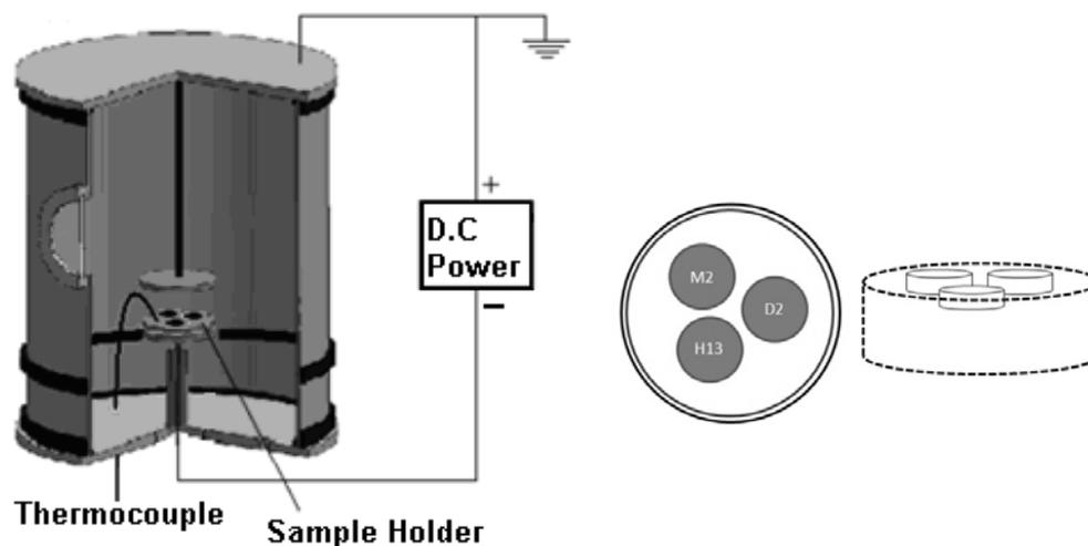
a) **Figure 1.** Schematic diagram of a) the nitriding chamber<sup>(6)</sup> and b) the sample holder used to nitride three different steel samples simultaneously.
