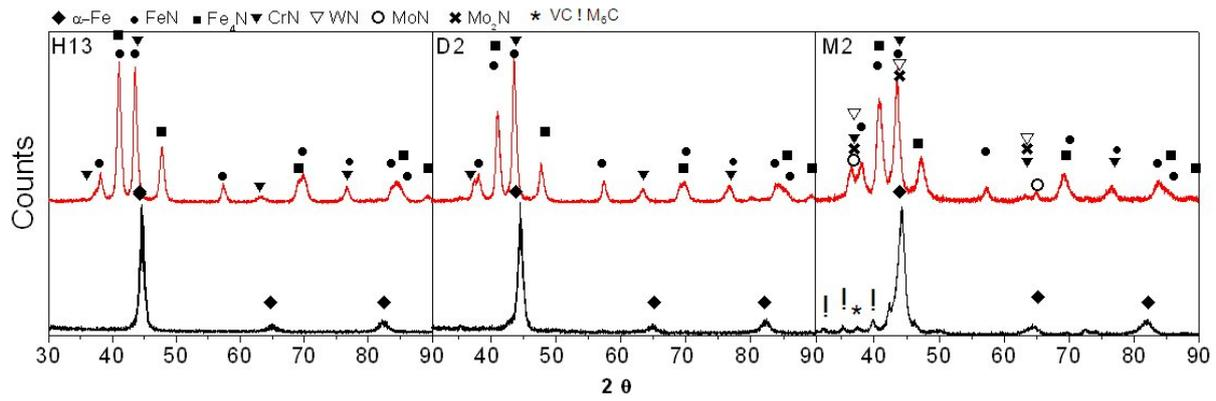
**Figure 3.** GIXRD with 8° incidence of AISI H13, AISI D2 and AISI M2 steels, before (black) and after nitriding (red).
