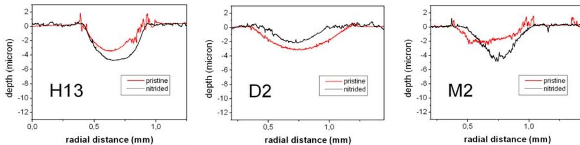
**Figure 8.** Wear profiles of the steels, before and after nitriding
