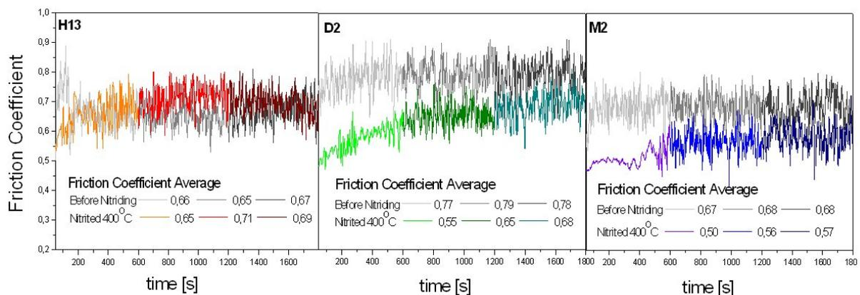
**Figure 7.** COF versus time (in seconds) before (grey scale coded) and after nitriding (color coded) of the steel samples. Mean values of each stage are inset.
