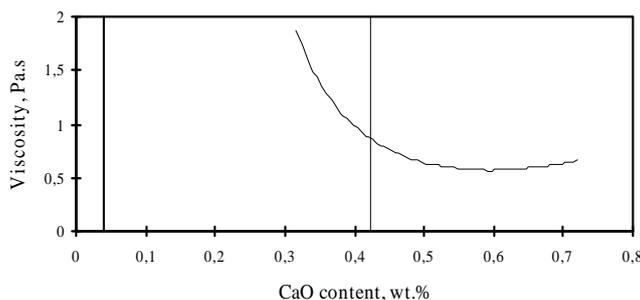
**Figure 4.** Viscosity at 1,450°C as a function of CaO content for the slag with 8 wt.% MgO and 20 wt.% Al<sub>2</sub>O<sub>3</sub>.
