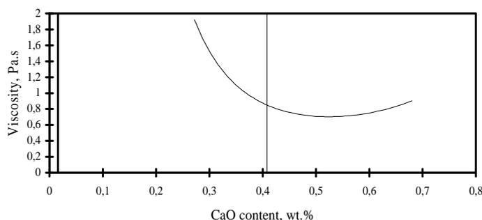
**Figure 5.** Viscosity at 1,450°C as a function of CaO content for the slag with 12 wt.% MgO and 20 wt.% Al<sub>2</sub>O<sub>3</sub>.
