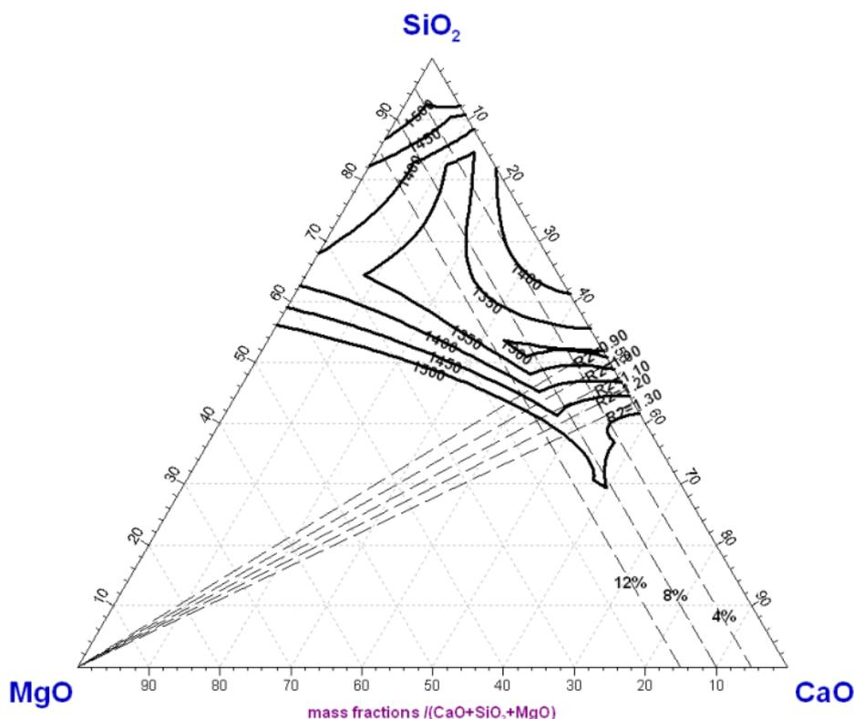
Figure 1. (a) Isotherms of the quarternary slag system with 20 wt.%  $\text{Al}_2\text{O}_3$  (by using database FToxid).
