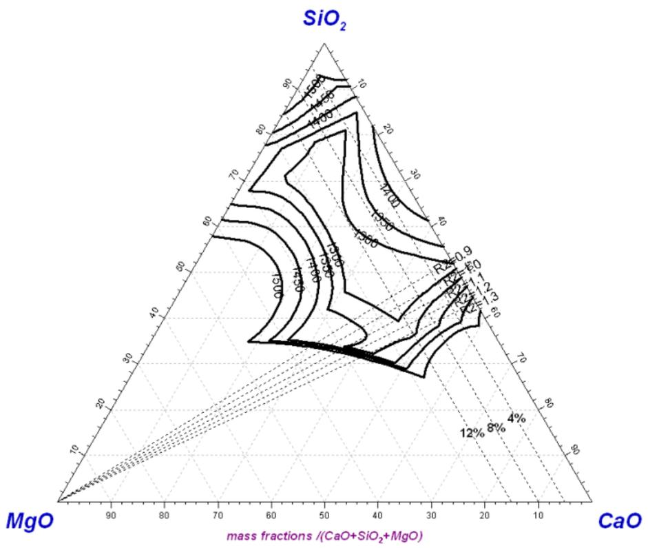
Figure 1. (b) Isotherms of the quaternary slag system with 20 wt.% Al<sub>2</sub>O<sub>3</sub> (by using database Fact).
