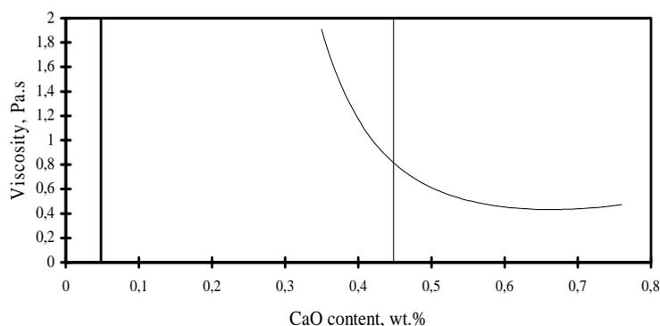
**Figure 3.** Viscosity at 1450 °C as a function of CaO content for the slag with 4 wt.% MgO and 20 wt.% Al<sub>2</sub>O<sub>3</sub>.
