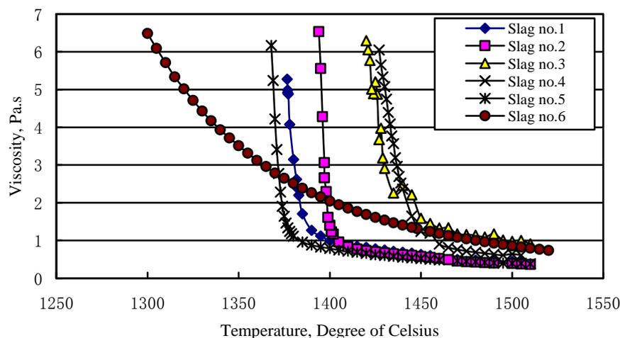
**Figure 6.** Viscosity as a function of temperature of the quarternary slag system with 20 wt.%  $\text{Al}_2\text{O}_3$ .
