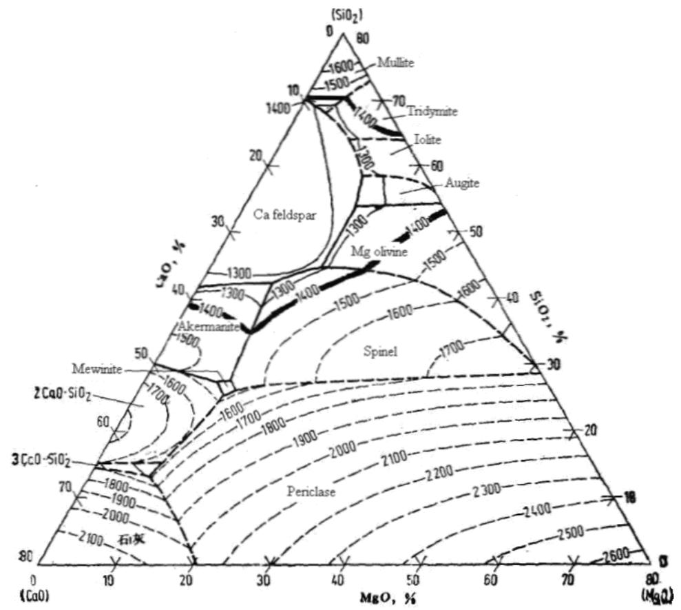
Figure 2. Measured Phase diagram of CaO-MgO-SiO<sub>2</sub> system with 20 wt.% Al<sub>2</sub>O<sub>3</sub>.
