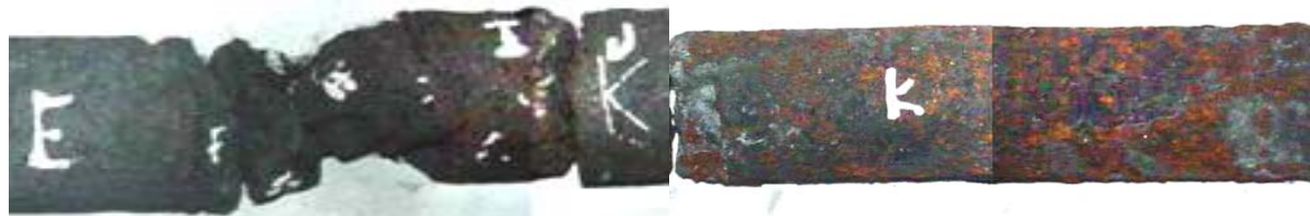
Figure 7. Cracked carbon impregnated with iron
