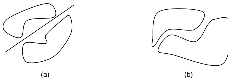
Figure 1. Examples of relationship: (a) Linearly separable patterns and (b) Non-linearly separable patterns.
