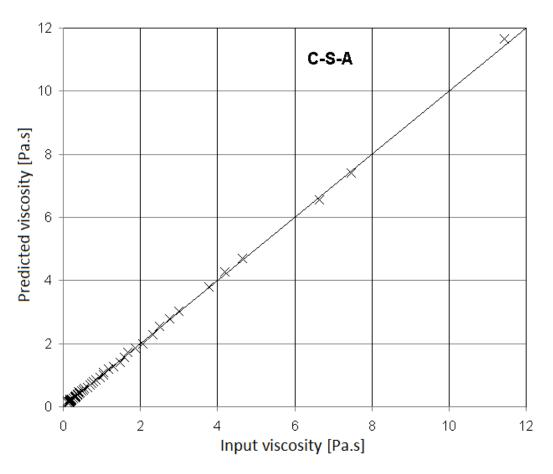
Figure 1. Predicted viscosity values as a function of the input values, C-S-A system
