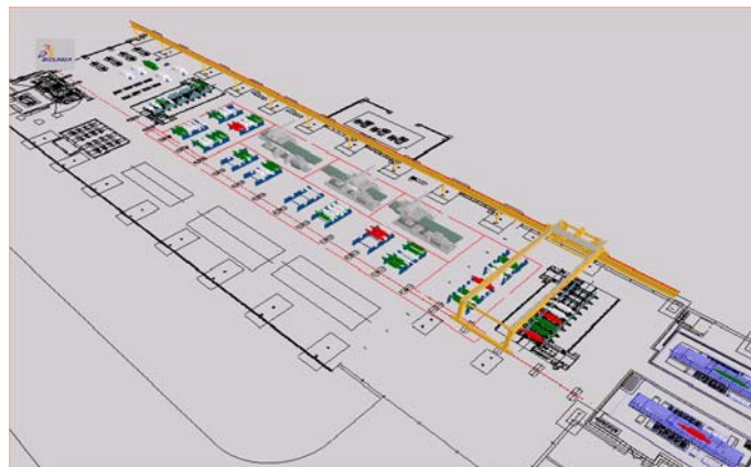
Figure 3: Virtual roll shop showing a fully automated work cell.
