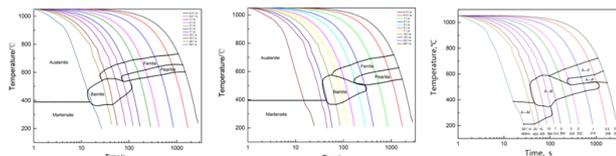
**Figure 9.** CCT curve of three sets simulation experiments
