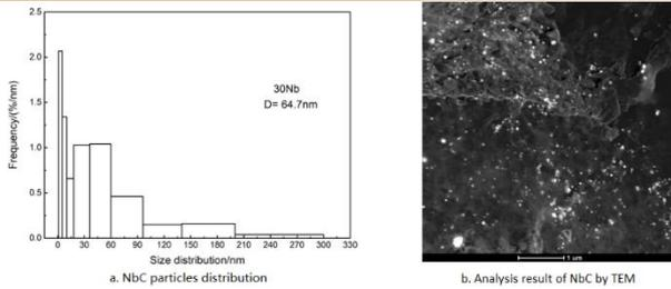
**Figure 11.** Analysis result of Nb-bearing reinforcing bar with TEM
