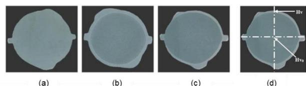
**Figure 1.** Metallography picture of the cross-section of a rebar
