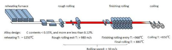
**Figure 3.** Typical layout of hot rolling strip and key temperature parameters
