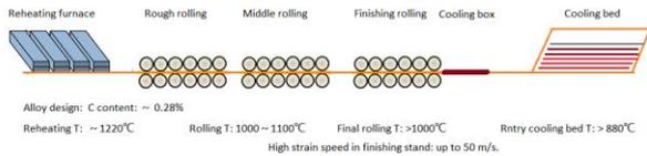
**Figure 4.** Typical layout of bar production line and key temperature parameters
