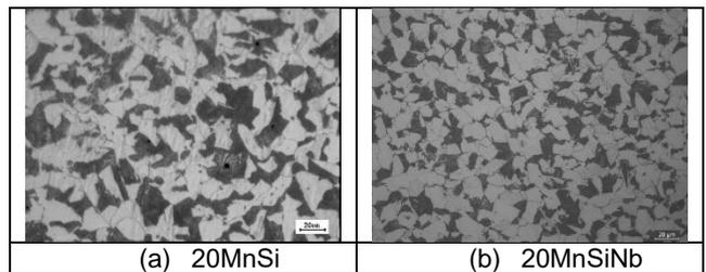
**Figure 10.** Comparison of optical microstructure between 20MnSi and 20MnSiNb
