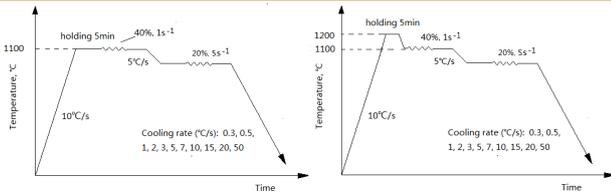
**Figure 8.** Schematic of CCT simulation tests
