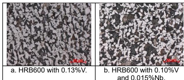
**Figure 5.** Optical microstructure and HRB600
