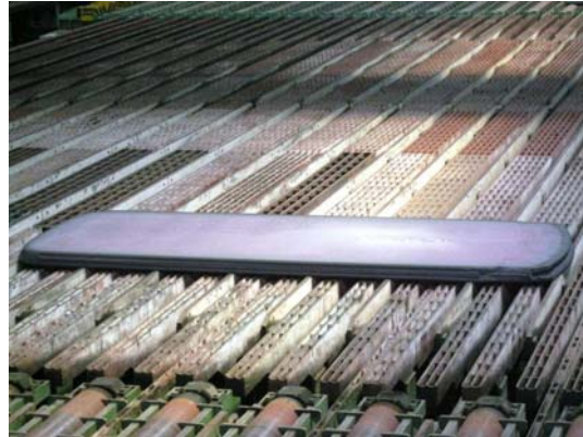
Figure 10. Final plate on the cooling bed.
