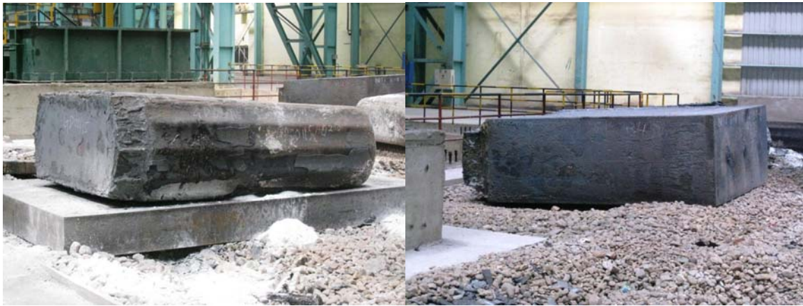
Figure 1. (a) Tapered ingot; (b) Cuboid ingot.
