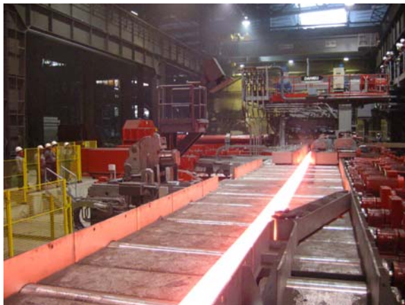
Figure 6. SCC stand in operation at VAS
