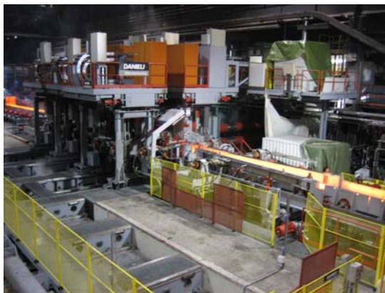
Figure 2. SCC stand in operation.
