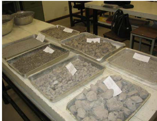
Figure 1. Steel slag in granulometric fractions 0-32mm
